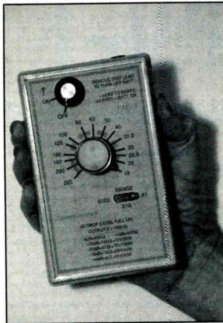
The PAG-1 is a 9V handheld battery powered portable audio generator.
