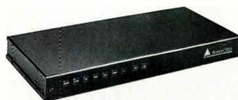
Audioaccess' PX-6 multi-room remote controller.
