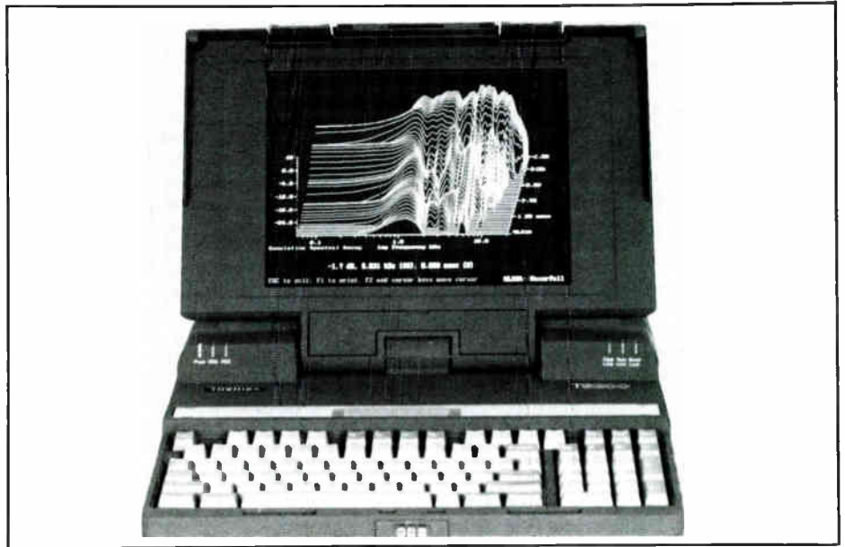
MLSSA Acoustical Measurement system running in a Toshiba T5200 laptop.
