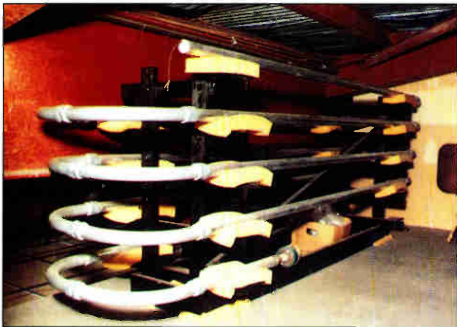
Pre-digital time delay, circa 1950. One hundred and twenty feet of metal tubing was used to solve the problem of under-balcony delay.
