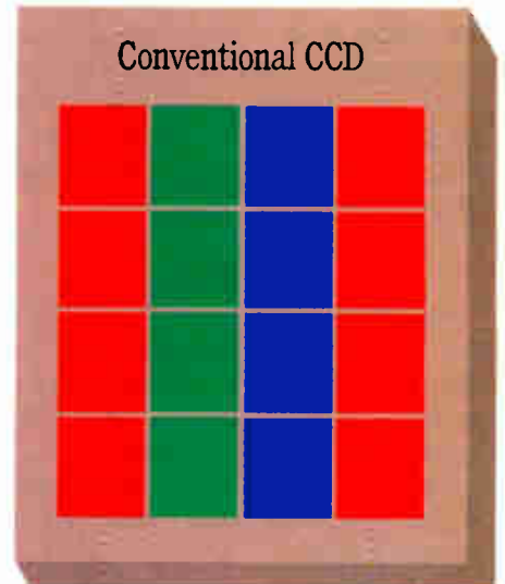
Conventional CCD: Red, green, blue "stripe" sensors can't resolve fine color detail, suffer from "channeling" when exposed to hot spots of light.
