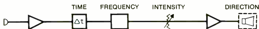
Figure 3: Basic channel for reflected energy system, which show the components that simulate D.I.F.T.
