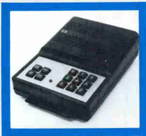
F/B Ektacom's hands-free digital intercom uses a simple, three-pair cable that circulates between stations.
