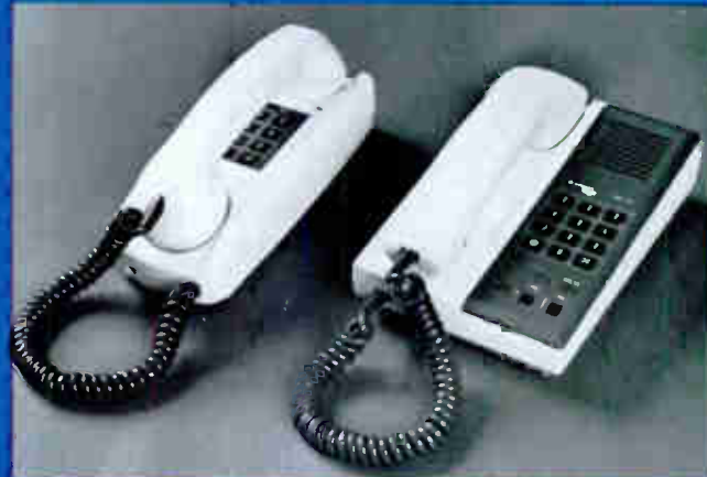
YKX combination speaker-phone intercom by Aiphone is a microprocessor-based intercom.
