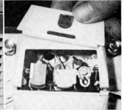
Left: tape motion controls are grouped at front center on top of recorder. Record safety interlock is at right rear with ornamental matching piece to the left. Center: battery condition and record volume meter is to left of volume control wheel. Right: head covers may be removed for cleaning heads. This photo shows rear cover removed; front cover also is removable.
