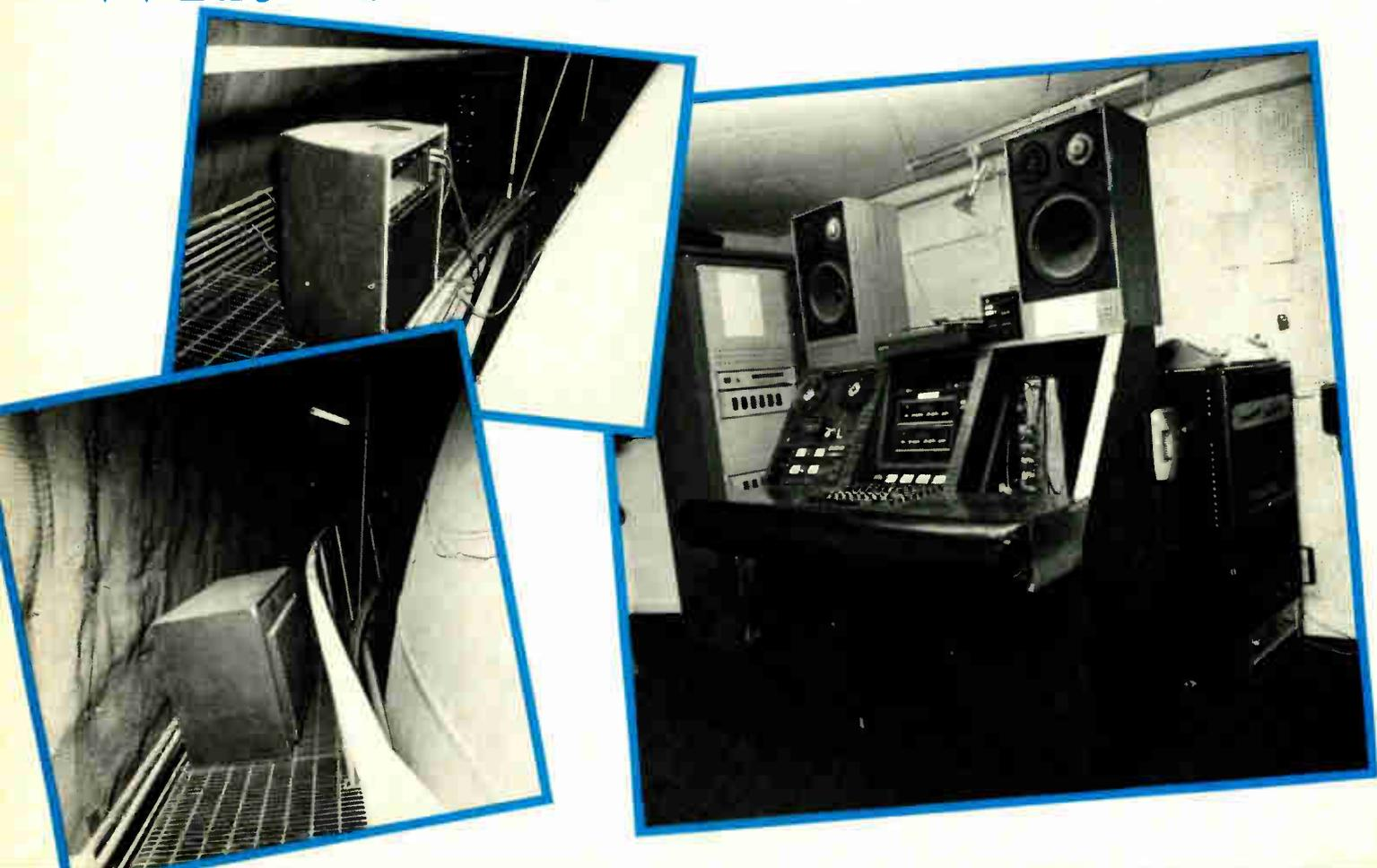
To counter this, a clever multi-speaker arrangement is employed, with four channels of sound—two left and two right—placed at 90° points on the dome.
