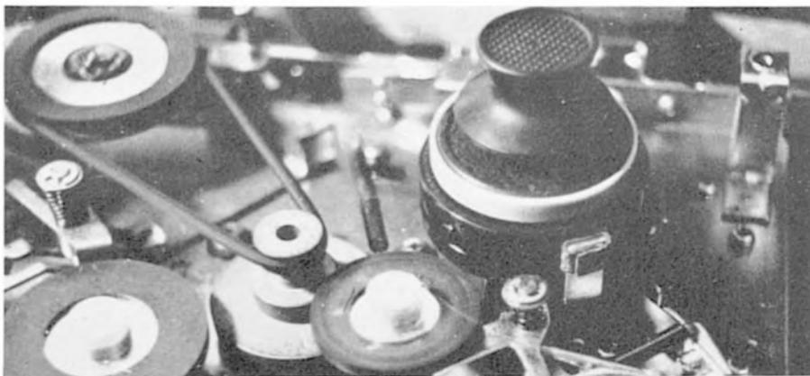
**Above:** One Sony version, where a combination of belt and pulley drive dictates clutch style. Basically a weight-dependent type but relying on the pulley drive for its efficiency.
