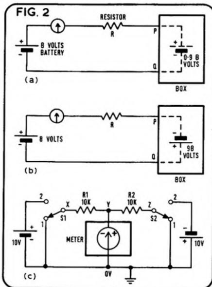
between P and Q of the same polarity as the battery B but with a voltage one tenth of B less—and the final result is a voltage of about 0.1B volts across the resistor. Normally we would expect that a battery of 10V connected in series with a resistor of 10K produces a current of 1 mA. However, instead of 10V drop across R, we have 1V drop. In other words, we have made a 10K resistor look like a 100K resistor.
