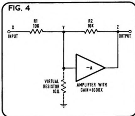
the value of R2 divided by the amplifier gain. Since this is the case, we could make this resistor any value we like by altering the amplifier gain and R2. The value of the imaginary resistor is not affected by R1. Negative feedback has reduced the input impedance of the overall system to a value of our own choosing. We can, thus, make it 600 ohms if we like and this can be used as the load for a microphone.
