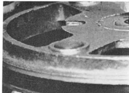
**Lower right:** Excessive wear. The vulcan pads that transmit torque from lower to upper sections of this Philips clutch are worn almost flat. They should be domed.
