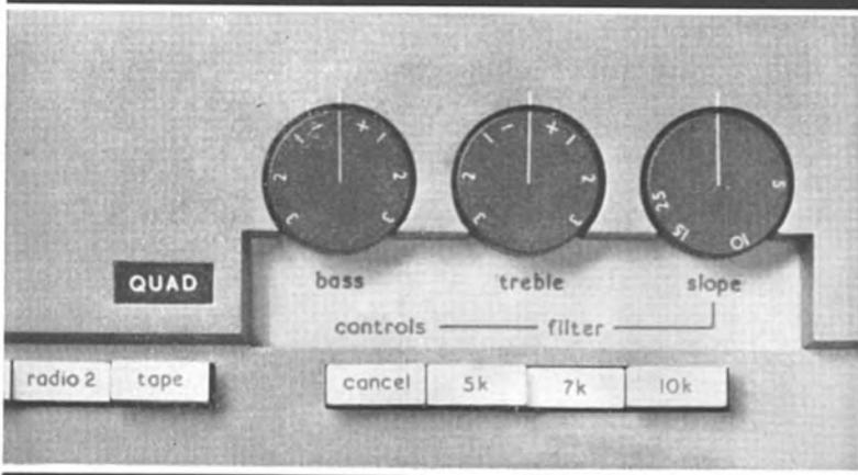
Set up a QUAD 33 with +1 on the treble control, and you will obtain a response precisely defined; readily and accurately repeatable. This response has a shape rather different from most run of the mill tone controls and there are, as you may guess, good reasons for this.
