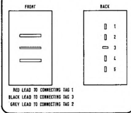
FIG. 2 TAPE CASSETTE SHOWING CASE CUT-AWAY
