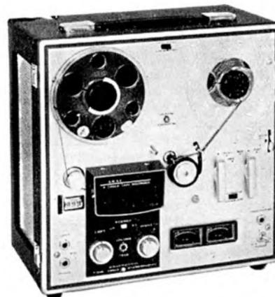
**AKAI I710W Stereo Tape Recorder (left).** The Shield Type Head for High S/N Ratio. 4-track stereo/monaural recording and playback. 3-speeds (1½, 3½ and 7½ ips (15 ips optional)). Automatic shut off. Pause lever. Tape cleaner. Tape shifter in fast forward/rewind operation. 4 hours maximum stereo recording capacity with a 1,200 feet tape. DIN jack, Stereo headphone jack. 3-digit index counter with reset button, VU meters. Finely oil-finished wooden cabinet. List price £109. Our price £89 10s.
