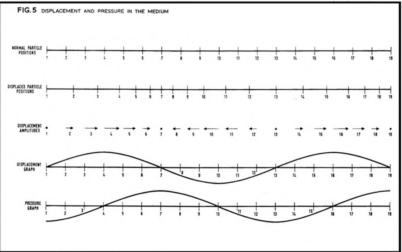
It should be noted that the horizontal axis indicates distance (not time) and the pressure wave *leads* the displacement wave by 90°. (The waves are taken to be travelling from left to right, as in fig. 4.)
