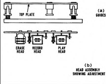
head is replaced, the only way of making sure is to experiment with shims between the head and mounting plate. Record/play heads have more scope for screw adjustment.
