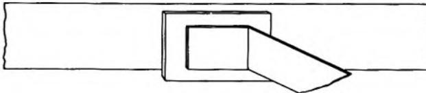
FIG. 4 OUTER TRACK FADING AND INNER TRACK CROSSTALK DUE TO HEAD MISALIGNMENT
