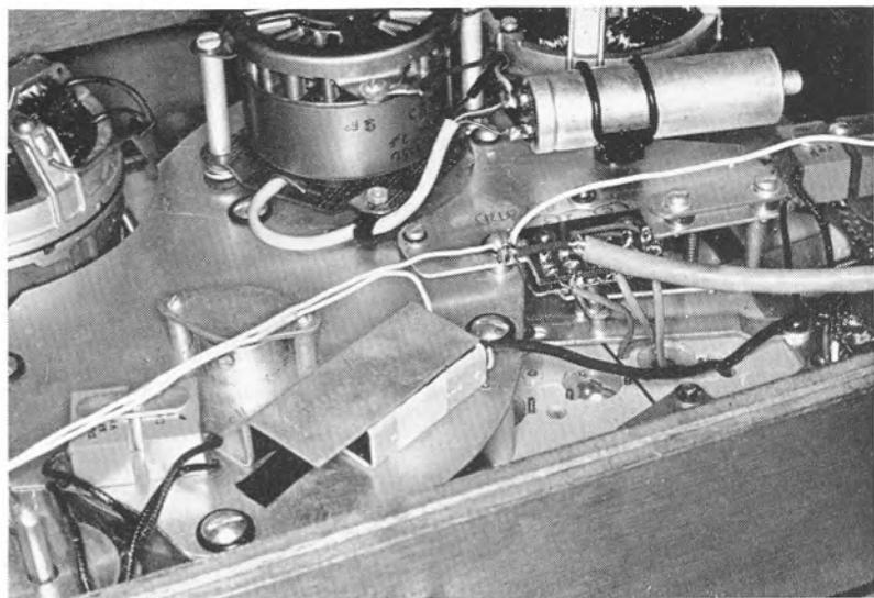
Fig. 3. Battery mounting beneath deck.
