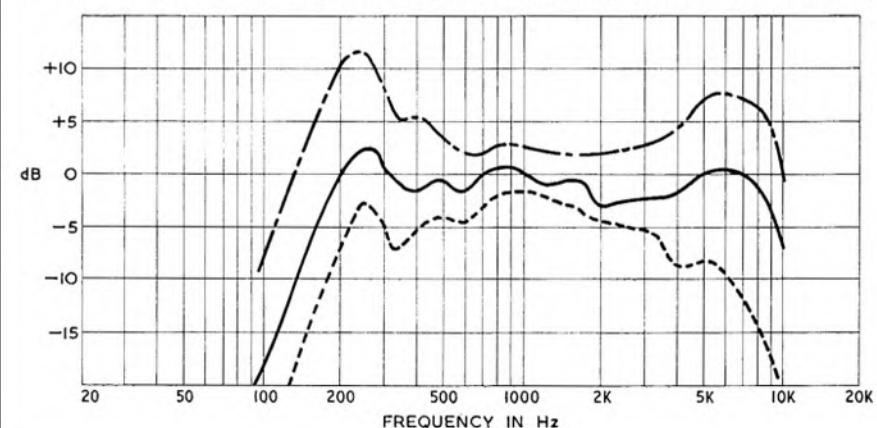
FIG. 5 SONY TC-530 MICROPHONE RESPONSE (200 OHMS IMPEDANCE)
