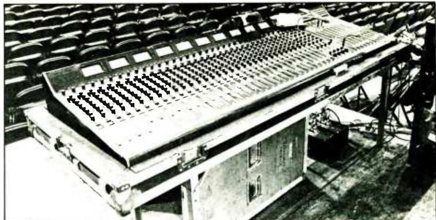
Figure 6: Midas 32-input PR Series stereo house console. Effects and outboard units also located at the house mixing position include a Roland SRE555 Chorus Echo, GML/Nova Research Model 8045 five-way stereo crossover, GML/Nova Series II Dynamic Gain Control compressor-limiters, Eventide H949 Harmonizer, Orban Model 622B parametric equalizer, Nakamichi 550 cassette and a ReVox B77 stereo reel-to-reel.
