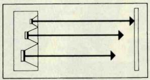
**Conventional Driver Mounting** in a common flat baffle. Smaller drivers have lower mass and shallower cone surfaces. High frequencies arrive earlier than lower frequencies, harmonic overtones before fundamentals. This is time delay distortion.
