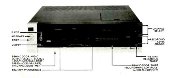
THE VHS CAMP has at last responded to the Beta Hi-Fi challenge with an improved VCR audio recording system of its own, not surprisingly called VHS Hi-Fi. The Hitachi VT-88A is the first VCR using the new system to come into our hands.
