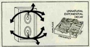
Diffraction Delay Distortion. In conventional speaker systems, sound wave energy radiates across the speaker baffle to the edges of the cabinet and is diffracted. These secondary signals create unnatural exponential decay and destroy clarity and spaciousness.
