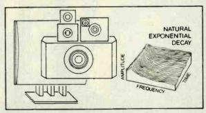
The Dahlquist Solution. In the DQ-10, the staggered baffle plates are sized to minimize diffraction. It is as though the drivers are mounted in free space with no nearby obstructions to distort the pure sound source. Sound decays naturally.
