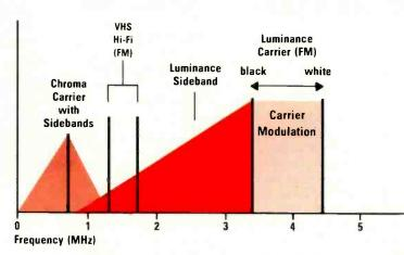
FIG. 2. THE VHS RECORDING format has no convenient space for the audio FM carriers. VHS Hi-Fi, therefore, uses only a single carrier each for the left and right audio channels (at 1.3 and 1.7 MHz, respectively) and minimizes crosstalk and video interference by using differently canted audio and video recording heads.
