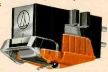
for good reason. Our unique, patented\* Dual Magnet construction provides a *separate* magnetic system for *each* stereo channel. A concept that insures excellent stereo separation, while lowering magnet mass. And the AT12XE features a tiny  $0.3 \times 0.7$ -mil nude-mounted elliptical diamond stylus on a thin-wall cantilever to further reduce moving mass where it counts. Each cartridge is individually
