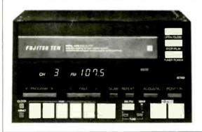
Most of the prototype car CD players we've seen are dedicated devices—that is, they complement existing car-stereo systems by adding CD playback. This Fujitsu Ten unit goes one better by combining an AM/FM tuner and CD player in one chassis, with some multipurpose controls. And models that add tape playback should appear soon.
