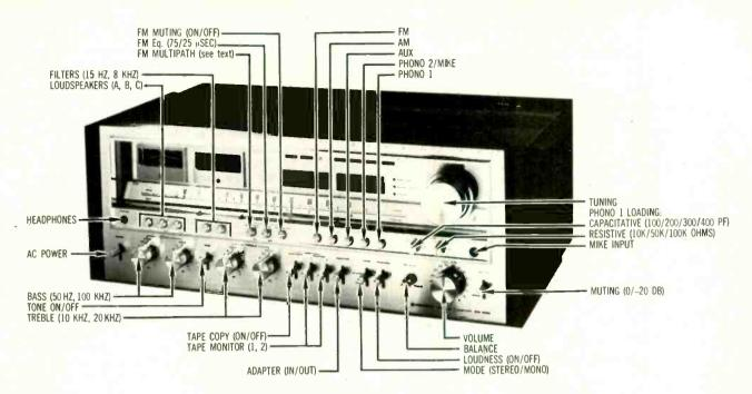
reaches + 13 and -141/2 dB at the lowest frequencies, hinging from a 400-Hz turnover point. To this can be added the 5-position 50-Hz control that provides a spread of  $\pm$  3 dB at 50 Hz and +8 to -9 dB at 20 Hz. At the high end, the 10-kHz control reaches + 10 and -11 dB at 20 kHz from a 1.5 kHz turnover, and approximately ±5 dB additional is offered by the 20-kHz control. The loudness contour boosts both the bass and treble ends of the spectrum.
