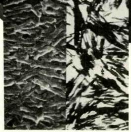
TDK SA tape surface (left) enlarged 30,000 times. TDK Super Avilyn particles (right) enlarged 20,000 times.
