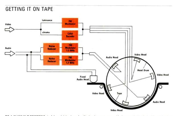
FIG. 3. IN VHS HI-FI RECORDING, the left- and right-channel audio signals are compressed (to be expanded in playback), modulated on separate FM carriers, and recorded via two audio-only heads mounted on the rotating head drum. The higher-frequency video information is then recorded over the audio. A stationary head records a standard audio track for compatibility with non-Hi-Fi VCRs.
