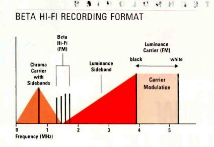
FIG. 1. BETA HI-FI'S four audio FM carriers (two each for the left and right channels) are sandwiched between the chroma and luminance signals. To make room for them, the luminance carrier is shifted up in frequency (in comparison to standard Beta) by 400 kHz, so that it ranges between 3.9 and 5.2 MHz.
