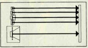
The Dahlquist Solution. With Phased Array<sup>™</sup> Mounting, drivers are positioned so that all frequencies (fundamentals and harmonic overtones) reach the listener at the same time. Musical sound is in phase.
