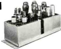
A novel and unique circuit design is employed to provide 50 watts of continuous power (100 watts peak) with amazingly clean, distortion-free reproduction. Frequency response extends from 20 to 20,000 cycles,  $\pm 1$  db, and from 10 to 100,000 cycles,  $\pm 3$  db. Distortion is less than 1% over the entire audible spectrum at full 50-watt output. Phase shift is negligible. High damping factor and other features contribute much to the outstanding listening quality of the 50 W-2.
