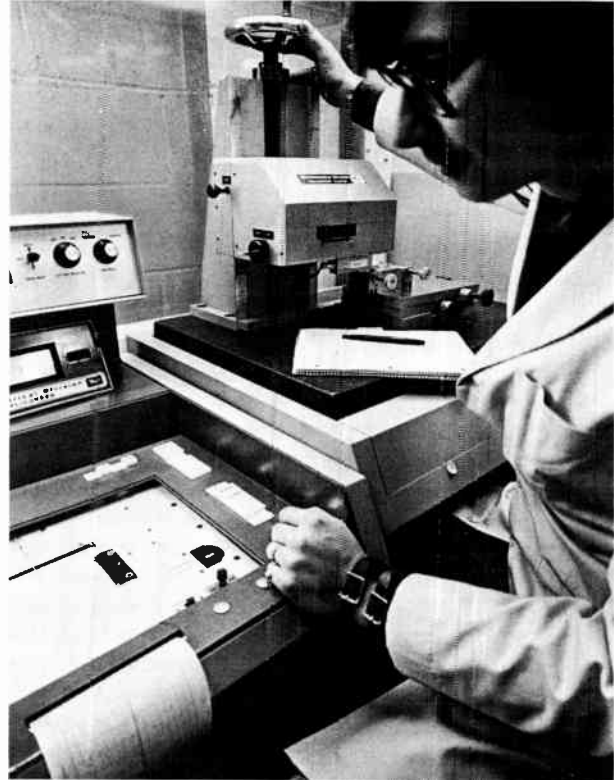
Precision surface analyzer measures tape smoothness profile and plots it on chart with a 1-millionth of an inch sensitivity.
