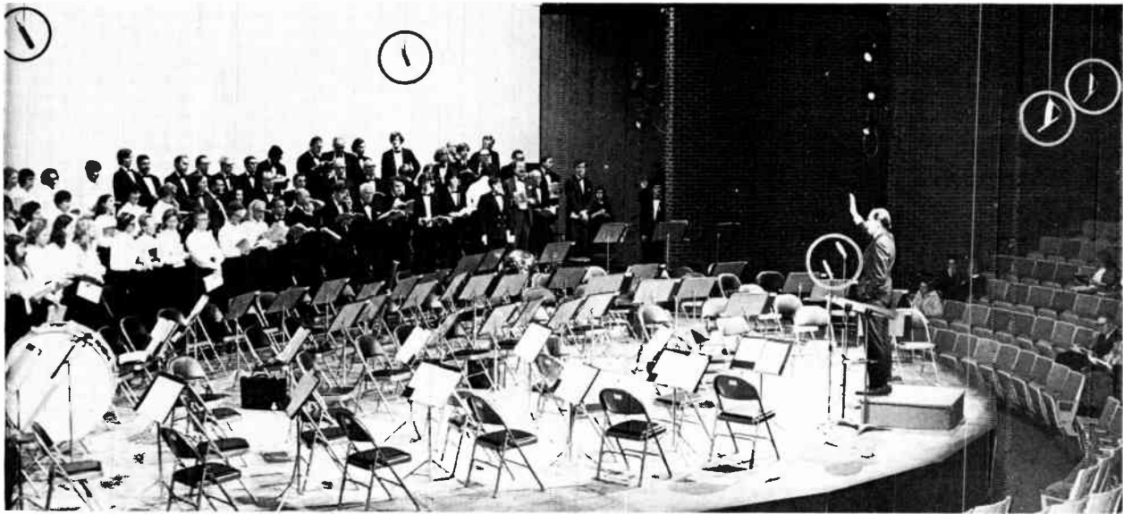
Fig. 3. Primary microphone placement photographed during a choir rehearsal. The two choir microphones are shown hanging from ceiling above the choir. The soloists' microphones are standing in front of conductor and the two front two of the four main microphones can be seen directly behind and above the conductor.
