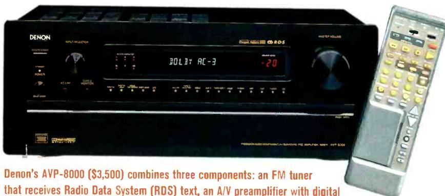
Denon's AVP-8000 (\$3,500) combines three components: an FM tuner that receives Radio Data System (RDS) text, an A/V preamplifier with digital signal processing, and a Dolby AC-3/Pro Logic surround-sound decoder.
