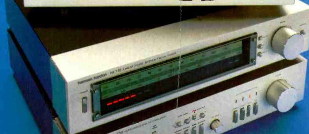
The hk710 High Technology phase locked analog tuner.
