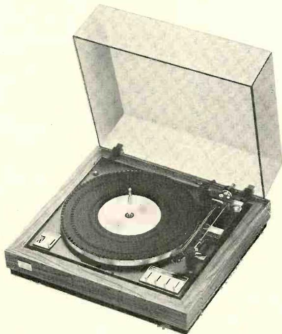
pered magnets that reduce the anti-skating force as the arm moves inward (since its head offset angle decreases simultaneously, less skating force is created at smaller playing diameters). The ball-bearing arm pivots are said to have 30 milligrams of friction in the horizontal plane and 20 milligrams vertically, measured at the stylus.
