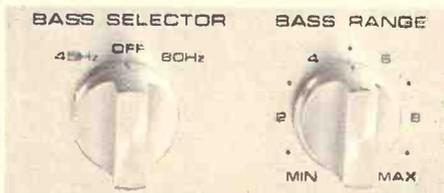
**Bass Extender.** A major exclusive feature of the RS1080 not found in any other receiver is our bass extender and bass range level control. At a flip of a control you can boost bass response up to 12dB at either 45 or 80Hz. Electrically tuned circuits assure sharp roll-off characteristics, and a tremendously
