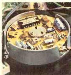
The Garrard DD75 delivers rock-steady speed with a DC motor, governed by an electronic servo system. It is totally immune to fluctuations in household current. The specifications are impressive: rumble  $-70\text{dB}$  (Din B), wow and flutter  $0.03\%$ . The same electronic system provides variable speed control,  $\pm 3\%$ , monitored by an easily-read, illuminated strobe.
