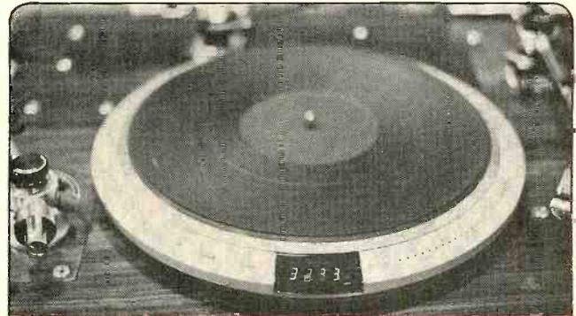
One of the quartz-lock turntables shown was this JVC model incorporating a digital speed readout in the rim surrounding the platter. Pushbuttons provide incremental speed changes.
