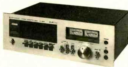
concentrically mounted and affecting both line and microphone inputs. When recording from microphones, an attenuator can be switched in when necessary to avoid overload of the mike inputs. The microphone jacks are located on the front panel along with a stereo-headphone jack.
