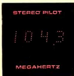
Four-digit LED readout is frequency-controlled (not synthesized). Accurate to 0.1mHz.
