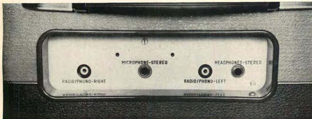
*EASY ACCESS* to input and output terminals is desirable. The Norelco 400 has recessed panels that enable connections to be made conveniently.
