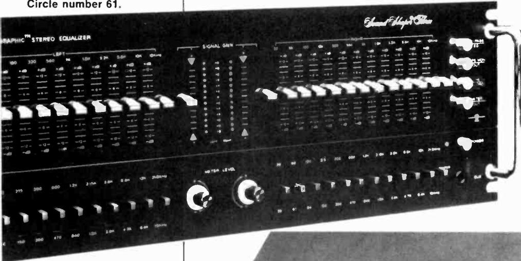
Sansui's SE-7 is a straight-forward 10-band graphic equalizer with  $\pm 12$  dB control over each of the bands. With the controls flat the frequency response is  $+0/-1$  dB from 10 to 100 kHz. It allows the user to compensate for system short-comings. Price: \$300. Circle number 89.
