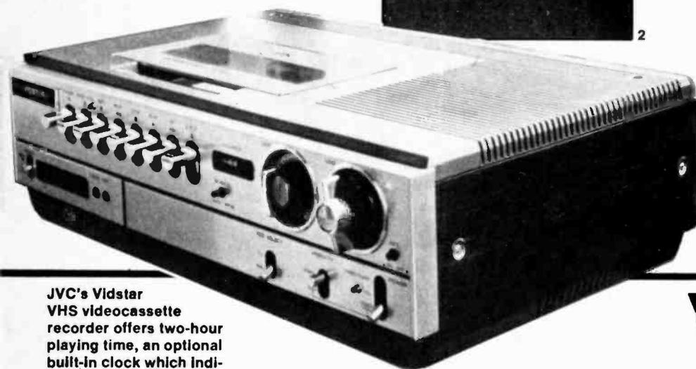
JVC's Vidstar VHS videocassette recorder offers two-hour playing time, an optional built-in clock which indicates time on a 24-hour basis. Its price: \$1050. Circle R. S. No. 148 to obtain further details.
