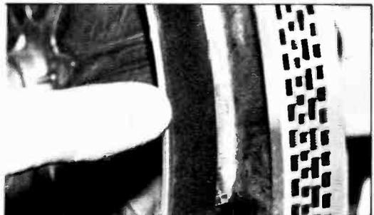
Here's a look at the magnetic deposit on the inside drive rim of an electronically-controlled turntable. Making an all-out effort to keep skin oil, etc. off it during assembly will prevent this.
