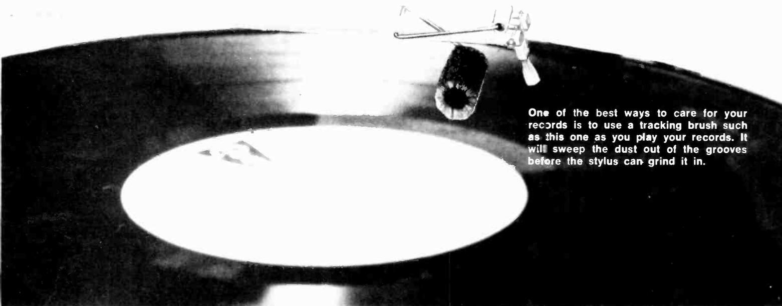
One of the best ways to care for your records is to use a tracking brush such as this one as you play your records. It will sweep the dust out of the grooves before the stylus can grind it in.
