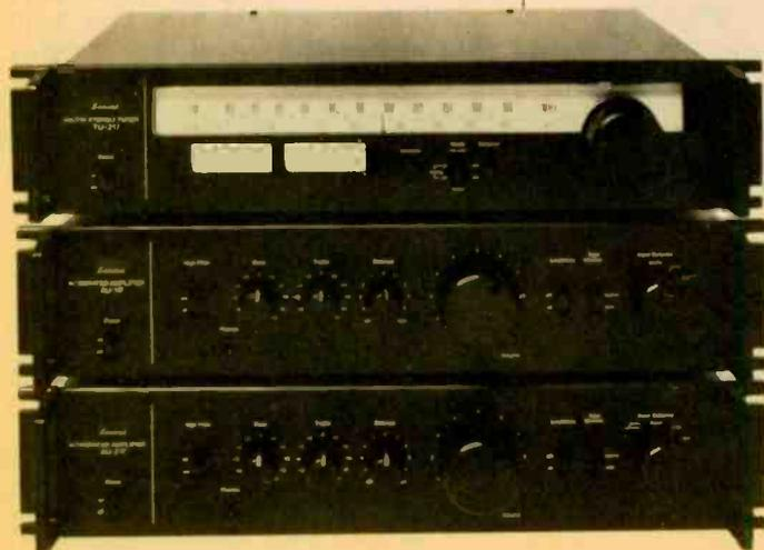
Sansui offers 3 new pieces: the TU-217 tuner (top) for \$175 (S/N: 71 dB); the AU-117 integrated amp (\$160) offering 15 wpc; and the AU-217 integrated amp with 30 wpc with less than .06% THD (\$190). #89.
