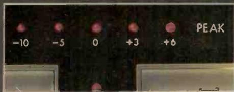
5 LED peak level indicators help eliminate distortion.
