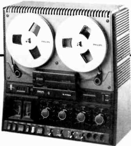
Philips N 4504 is a three-head, three-motor tape recorder which sells for \$450. Its signal-to-noise spec is 60 dB or better at 7½ and 3¾ ips. It accommodates 7-Inch reels. Circle Reader Service No. 84.
