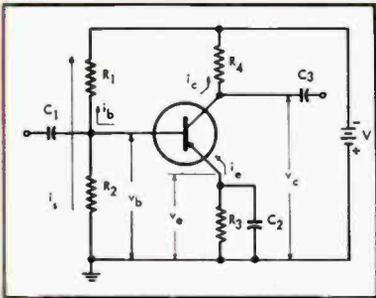
The problem of building stable transistor amplifiers hinges on the stabilization of the individual stages. See page 47 for the details.
