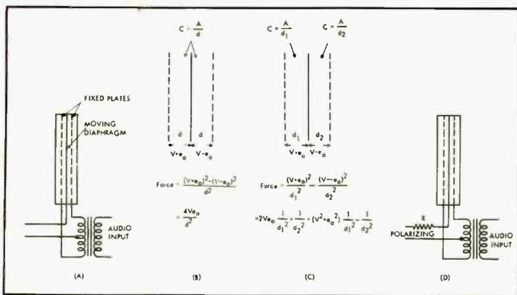
Fig. 1. The development of the distortionless push-pull electrostatic loudspeaker unit: (A) the basic arrangement with its drive unit; (B) this produces a linear driving force on the diaphragm, provided the diaphragm does not move; (C) when the diaphragm moves, the driving force becomes non-linear; (D) preventing the charge flow, mentioned in the text, by means of the resistor R, eliminates, or reduces, this non-linearity of driving force.
