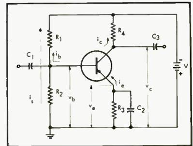
Fig. 2. By the addition of the voltage divider  $R_1$ - $R_2$ , the potential of the base is held fairly constant even though the emitter current may change appreciably.
