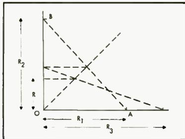
Fig. 3. Construction for three resistances in parallel.
