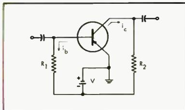
Fig. 1. Typical circuit for a low-power transistor as shown in many of the experimental applications. No provision is made for stabilization.
