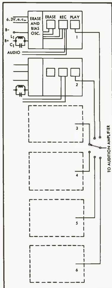
Fig. 2. Block diagram of connections to play heads of six recorders to permit audition of any one of them at will.
