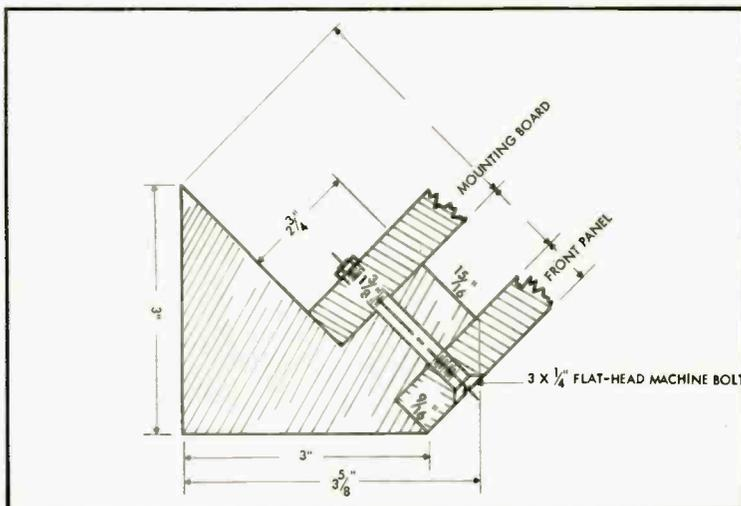
Fig. 4. Details of the front panel, speaker mounting board, and the hardwood corner post to show how the front corner of the cabinet is assembled.
