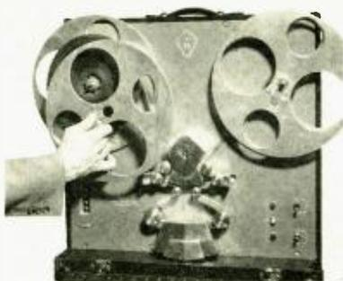
ment, Stencil-Hoffman Corporation, 921 N. Highland Ave., Hollywood 38, Calif., has announced detachable-flange reels for 16-, 17.5- and 35-mm film. The 1200-ft. reel has a removable flange which allows the raw stock to slip over the reel, after which the flange is secured in place by a half turn to a locking position. The reel is made of aluminum so that magnetic film can be handled safely. Further information will be mailed on request. **D-11**
