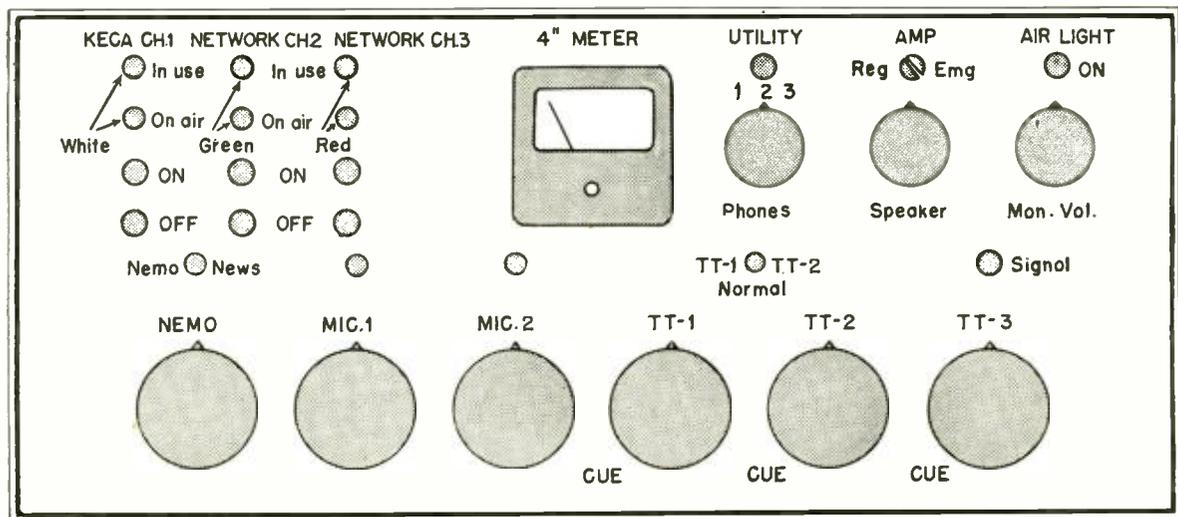
also puts the VI meter at an angle of best visibility to the operator. Thus, after having laid out the panel on cross-section paper until a satisfactory arrangement is obtained, the next step is to draw the panel layout accurately and to dimension all the mounting holes. Attention must be given to clearance between each part to make sure there is sufficient room for wiring.
