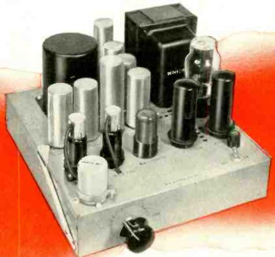
**Monitoring Amplifier (Type BA-4A)**—Designed for operation at microphone levels. High output of 12 watts is sufficient to drive several speakers or, in some applications, a recording head. Other uses include application as line amplifier for portable and mobile transmitters. *High gain:* 105 db. *Low noise level:* -20 db (with maximum gain); -40 db (with minimum gain). *Low distortion:* less than 3% at 12 watts. *Frequency response:* ±2 db, 30 to 15,000 cycles.
