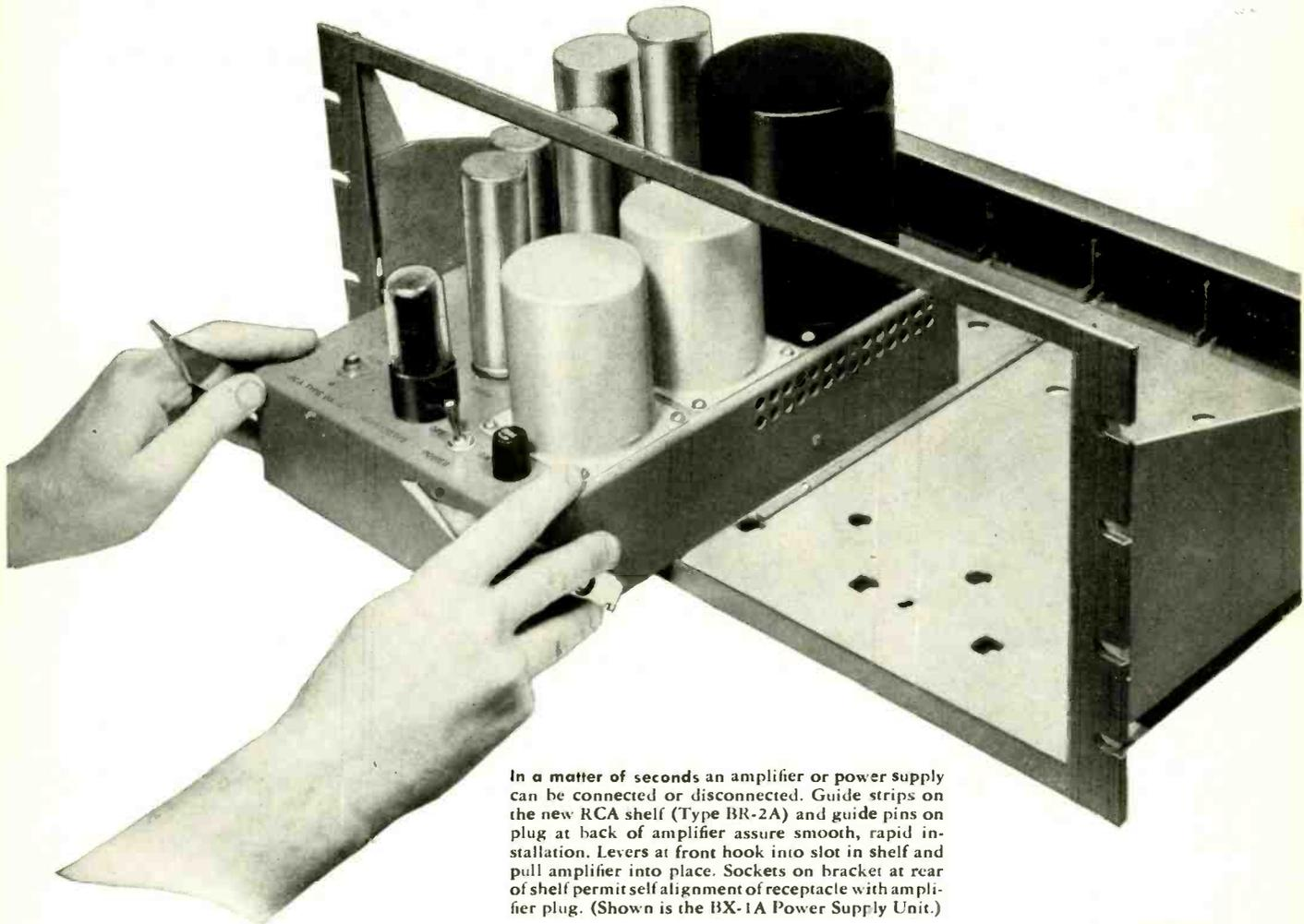
In a matter of seconds an amplifier or power supply can be connected or disconnected. Guide strips on the new RCA shelf (Type BR-2A) and guide pins on plug at back of amplifier assure smooth, rapid installation. Levers at front hook into slot in shelf and pull amplifier into place. Sockets on bracket at rear of shelf permit self alignment of receptacle with amplifier plug. (Shown is the BX-1A Power Supply Unit.)
