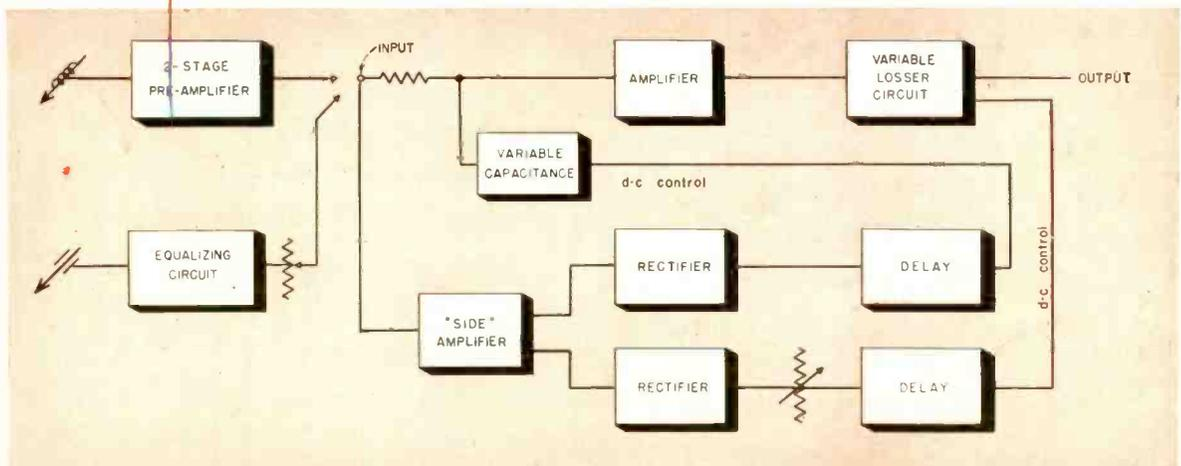
The signal channel is isolated from the preamplifier circuit in order that the effect of the scratch suppressor shall not be fed back to the side amplifier. Thus, the side amplifier is fed from the input circuit directly, while the signal channel is fed through a resistance network.
