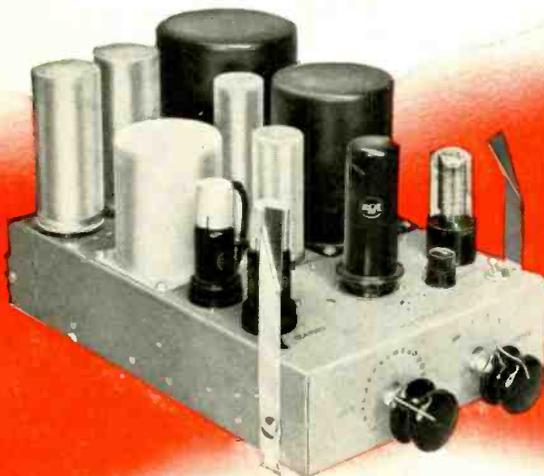
**Program Amplifier (Type BA-3A)**—one of the most versatile on the market. Ideal as a program, line, or booster amplifier; a high-level isolation amplifier; a cueing or monitoring amplifier, or a driver amplifier (for high-power recording amplifiers, etc.). *High gain:* 65 db for matching input, 27 db for bridging input. *Low noise level* (with maximum gain): -52 db. *Low distortion:* less than 0.5 to 1% rms, depending on output level. *Frequency response:* ±1 db, 30 to 15,000 cycles.
