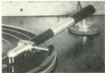
a new type spring loaded handle reducing stylus and record damage, arm resonance is less than plus or minus 1 db over the audio range of 40 to 15,000 cycles, and provides a proper stylus pressure of 22 grams for the GE and 15 grams for the Pickering.
