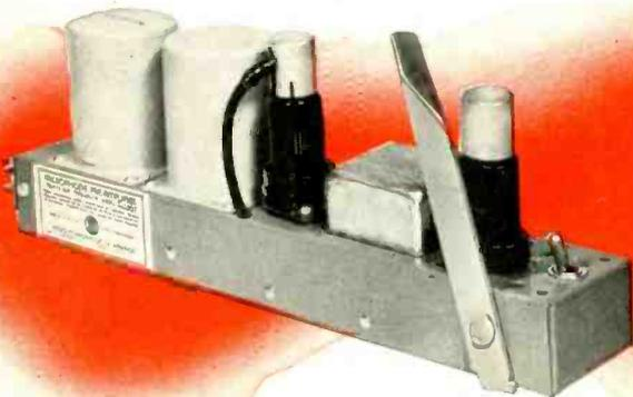
**Two-stage Preamplifier (Type BA-1A)**—ideal for use as a microphone preamplifier, turntable preamplifier, booster amplifier, or low-level isolation amplifier. *High gain:* 40 db. *High output:* +10 db. *Low noise level:* -80 db. *Low distortion:* 0.5% rms, 50 to 7500 cycles. *Isolation factor:* approx. 90 db; over 100 db with special Volume Control Kit. *Frequency response:*  $\pm 1$  db, 30 to 15,000 cycles. *Small size:* six units will fit on a 36-B or new BR-2A shelf!
