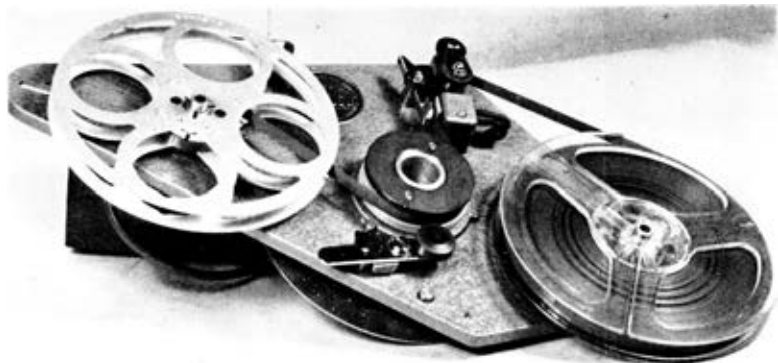
Above: The Gram-Deck—a novel design of deck which slips over the central spindle of a gramophone turntable to provide recording and playback facilities on tape. ( Andrew Merryfield Ltd. ) Below: A compact cabinet—tape, disc and radio are accommodated in this simple cabinet design—and there is storage space below.
