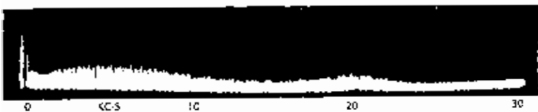
NOISE SPECTRUM FROM INSIDE GROOVE OF STANDARD 12" DECCA RECORD
