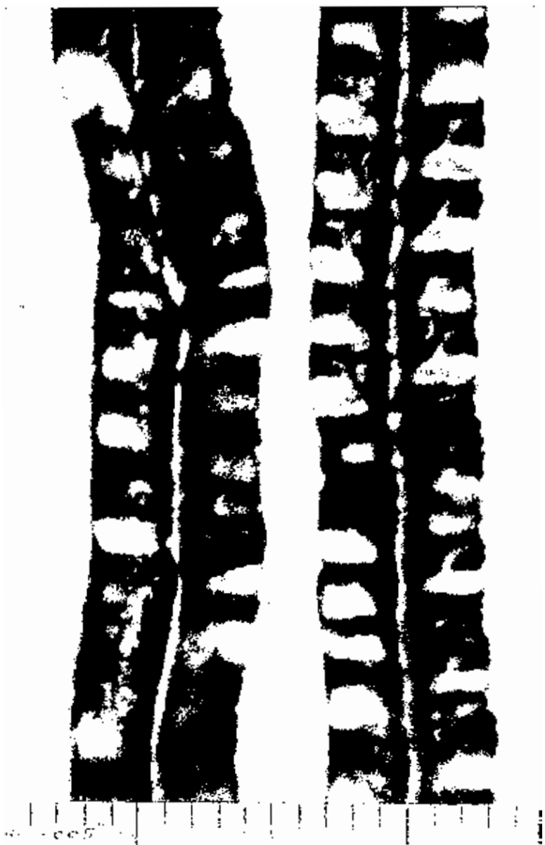
FIG. 73C.—Section of "Danse Macabre" record after 200 playings with crystal pick-up at 7\frac{1}{2} grammes.
