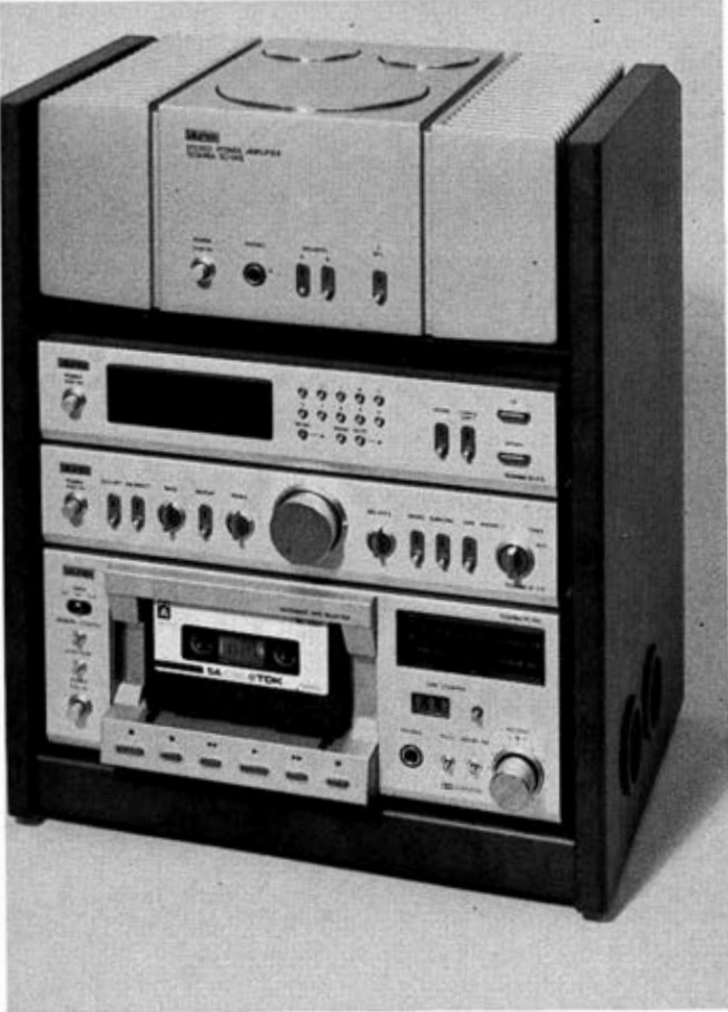
12 This mini hi-fi system has the power amplifier on top, with a separate preamplifier/control unit, radio tuner and cassette deck (Aurex Micro 15)
