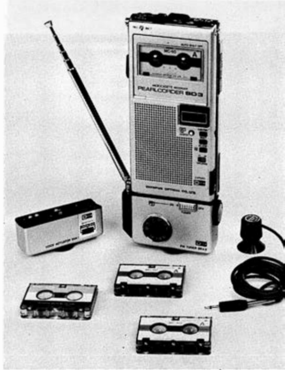
20 (above left) Exploded view of a typical cassette, showing the front pressure pad, loaded tape hubs and the spacer sheets which assist smooth spooling ( Photo Philips ) and 21 (above right) The microcassette system is being promoted as an even smaller successor to the compact cassette, with add-on tuners, etc (PearlCorder SD3)
