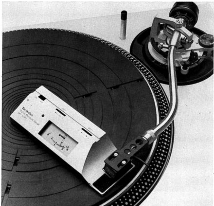
33 A separate pressure gauge can be used to check the pickup tracking force ( Technics SH-50P1 )
