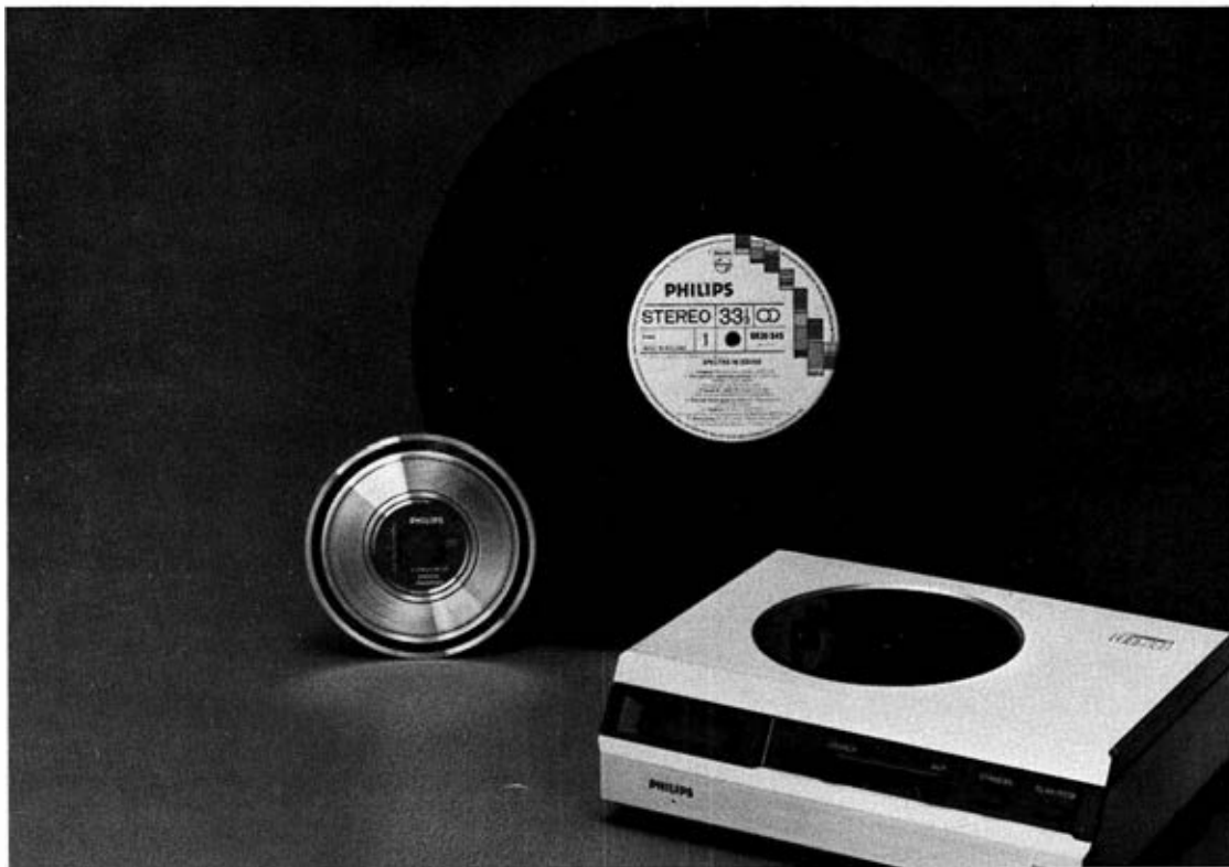
42 A Compact Digital Disc and its player unit, with a conventional LP record to show the relative size (Photo Philips)
