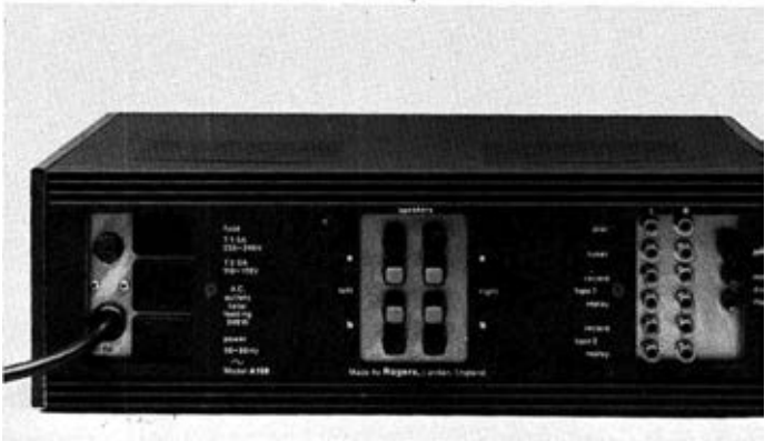
25 The back panel of the amplifier in Plate 24, showing push/hold loudspeaker terminals and phono-sockets for source inputs (Rogers A100)
