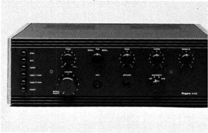
24 The front panel of a straightforward amplifier with push-button source selection and rotary knobs for filter, bass, treble, balance and volume (Rogers A100)
