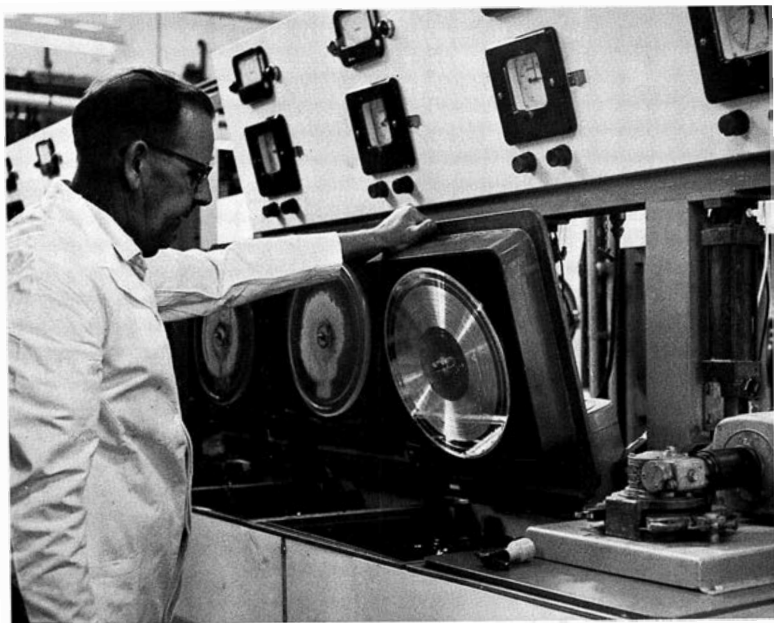
8 The metal stampers from which LP records are pressed are produced in electroplating baths ( Photo EMI )
