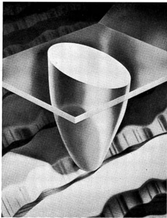
14 ( above left ) Magnified photograph of a cutting stylus during the making of a master disc, showing the thread of 'swarf' leaving the V-shaped groove ( Photo Cecil E. Watts ) and 15 ( above right ) Artist's impression of an elliptical reproducing stylus in a stereo record groove ( Photo Shure Bros )
