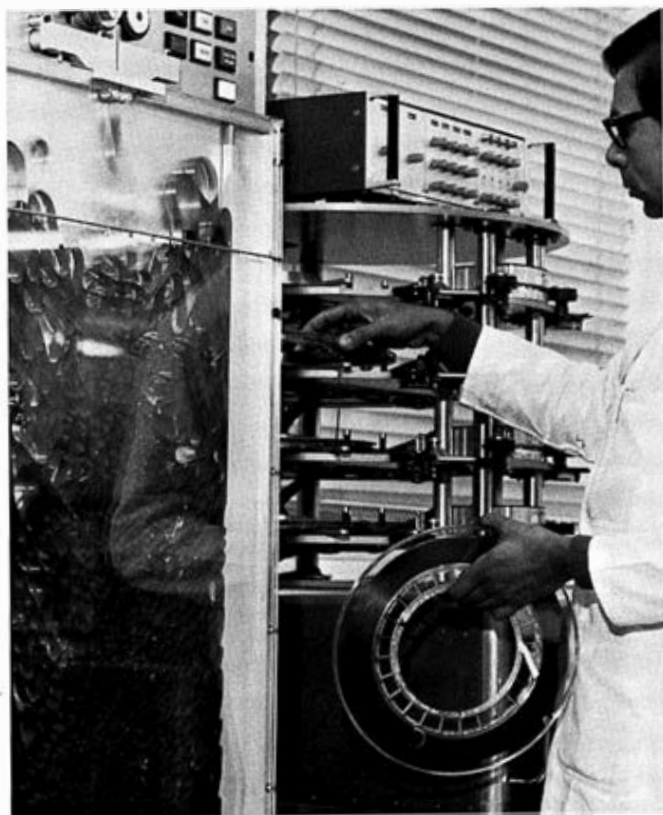
9 Musicassettes are duplicated at high speed on banks of 'slave' recorders from signals on the continuous-loop 1in master tape, visible through the glass panel on the left ( Photo Phonodisc )
