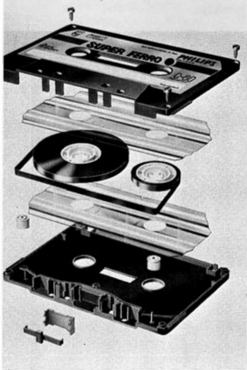
20 (above left) Exploded view of a typical cassette, showing the front pressure pad, loaded tape hubs and the spacer sheets which assist smooth spooling ( Photo Philips ) and 21 (above right) The microcassette system is being promoted as an even smaller successor to the compact cassette, with add-on tuners, etc (PearlCorder SD3)
