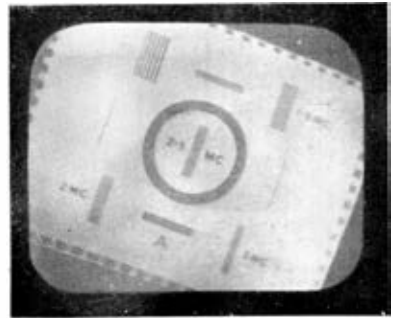
12—Picture tilted. Rotate deflector coil assembly until raster lines are horizontal
