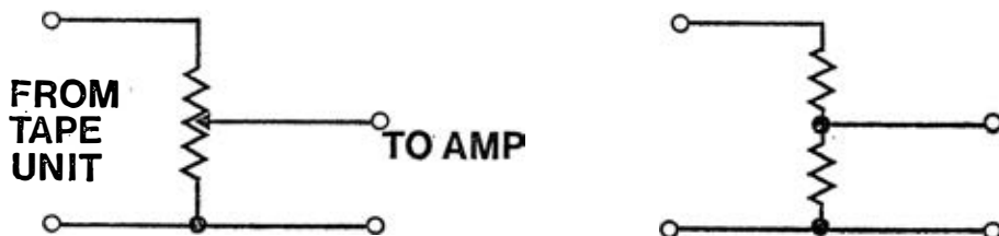
Use of potentiometer (one for each channel) to drop line output—see text.
