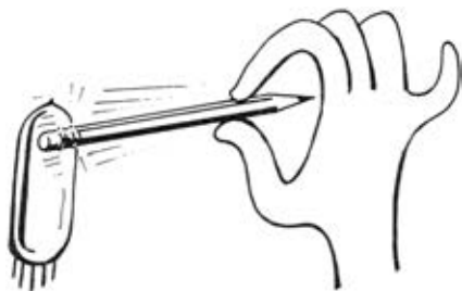
Fig. 503. Tapping a tube with the rubber end of a pencil.
