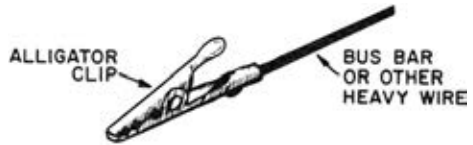
Fig. 1108. A self-clamping heat sink.
