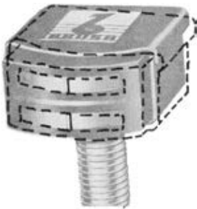
Fig. 612. Rotating a tape playback head about its vertical axis for possible improvement in bass response.
