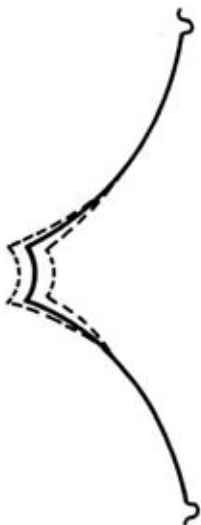
Fig. 7. Controlled flexure. At high frequencies the central areas of a curved cone move independently of the rest. The higher the frequency the smaller the active area. This thus serves as an effective high frequency radiator.
