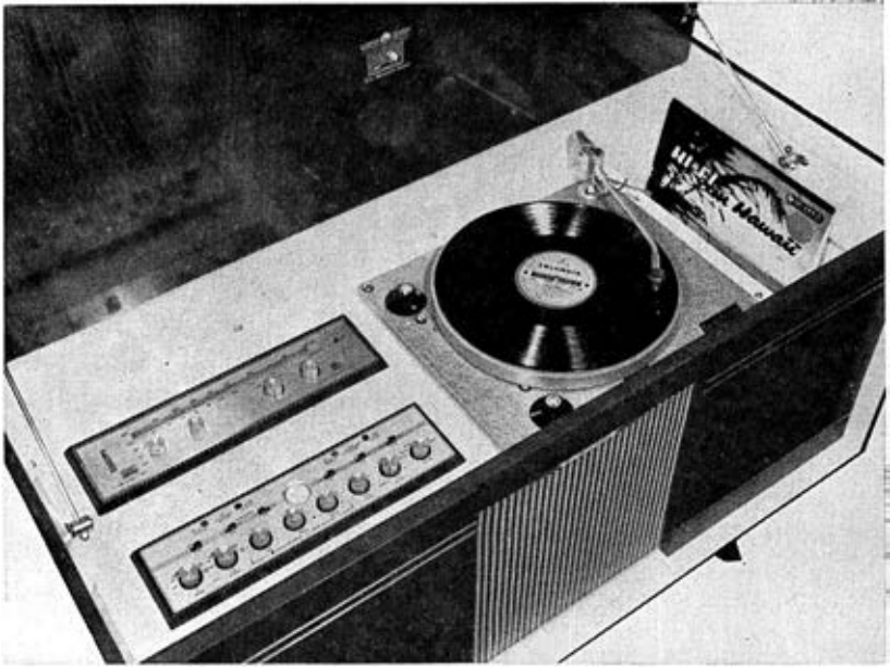
FIG. 3.—“HIS MASTER’S VOICE” MODEL 582 CABINET, FITTED WITH H.M.V. STEREO AMPLIFIER AND PICK-UP. A MATCHING RADIO TUNER UNIT AND A CONNOISSEUR TRANSCRIPTION UNIT ARE INCORPORATED. THE INSTALLATION IS COMPLETED BY MATCHED EXTERNAL LOUDSPEAKERS
