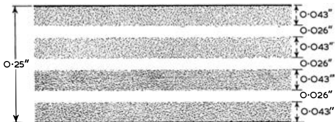
FIG. 8.—ARRANGEMENT OF FOUR TRACKS ON A \frac{1}{4} -IN. TAPE
