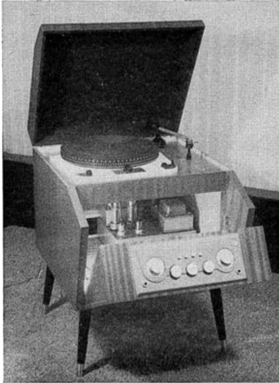
FIG. 2.—A NEAT GRAMOPHONE INSTALLATION The front can be lowered to give access to the amplifier.
