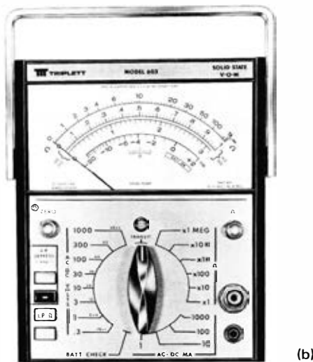
Figure 2-8. The loop resistance of a line is equal to the total resistance of the conductors: (a) representation of loop resistance; (b) loop resistance is measured with the ohmmeter section of a volt-ohm-milliammeter. (Courtesy Triplett Electrical Instrument Co.)
