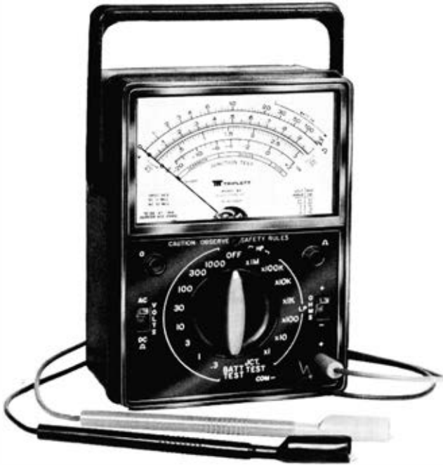
Figure 7-17. Solid-state VOM with high- and low-power ohmmeter functions. (Courtesy Triplett Electrical Instrument Co.)
