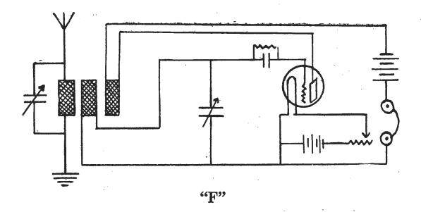
Circuit F.—Here we have a simple three honeycomb coil circuit. The coil between aerial and earth is the primary, the centre coil the secondary, the third coil, connected in the plate circuit, is the "tickler." In this circuit the coupling is varied by moving the primary coil while the oscillation strength is controlled by the "tickler."
