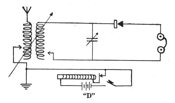
Circuit D.—This shows a simple loose coupler crystal receiver with a variable condenser shunting the secondary coil. The circuit also shows the arrangement for making a buzzer test for sensitive spots on a crystal. The key in the buzzer circuit is depressed and the operator listens in at the same time "searching" over the crystal with the catwhisker. The most sensitive spot on the crystal is reached when the buzzing noise is loudest in the 'phones.
