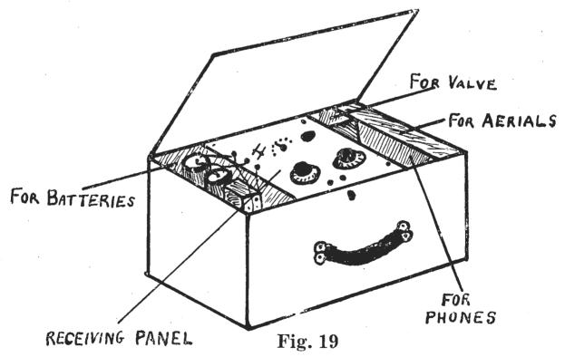
ters. A dry cell value is essential as the transportation of an accumulator, and its re-charging would be a cause of trouble. The dry cells for lighting the filament may be packed in the case, together with the "B" battery, and carried in any position without fear of accident.
