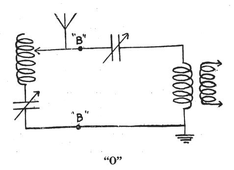
**Circuit O.**—Illustrates a circuit for tuning out an interfering station. The condenser "A" should have a capacity of .0005 mf. This circuit will only eliminate C.W. or I.C.W. signals of the frequency to which the coil and condenser are tuned. The portion to the right of "BB" represents any receiving set.
