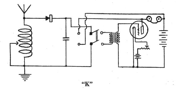
**Circuit K.**—This shows the "hook up" for a crystal detector and valve audio frequency amplifier. In the centre is seen a double pole double throw switch which is used to cut the amplifier in and out at will. Users of the crystal and valve combination will find this a handy arrangement.
