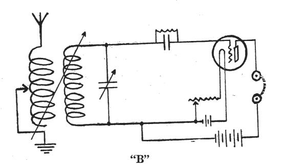
Circuit B.—This is a simple valve circuit arranged for use with a loose coupler. It is selective, but without regeneration.
