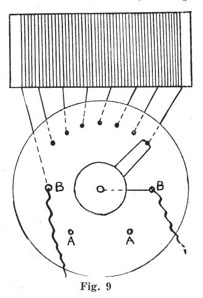
holes in each end are directly opposite one another. The holes marked "B" are made for flexible connections. The flexible wire mentioned in the list of parts is two stranded, and the strands should be separted to go one in each hole. One strand is connected inside the end to the tail left at the start of the secondary winding and the other to the switch arm.
