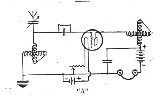
Circuit A.—A circuit in which the aerial and plate sections are tuned by variometers. The grid condenser should have a capacity of .0003 mf and that across the "B" battery and 'phones .01 mf. The aerial tuning condenser may be .0005.
