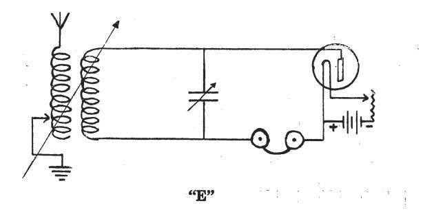
Circuit E.—This circuit shows the two electrode valve as a detector in conjunction with a loose coupler. The two electrode valve is rather more stable than a crystal but is not to be compared with the three element valve from the point of view of sensitivity.
