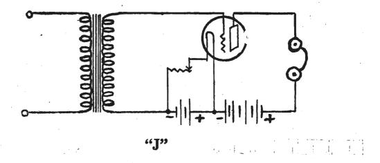
Circuit J.—This is a circuit for a single stage of audio frequency amplification which can be added to any detector. If being added to a single valve set the "A" and "B" batteries of the detector may be used but sometimes it is advisable to use a separate high tension battery. The input leads marked "A" are connected to the 'phone terminals on the detector panel.
