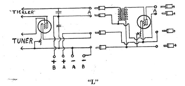
**Circuit L.**—This shows how a multi valve set may be connected up on the unit system. On the left is the detector panel and on the right a single stage of audo frequency amplification. Plugs and jacks are shown for adding more stages. When using one stage of amplification, on the detector alone, the 'phones should be plugged in at the pair of sockets marked "A."
