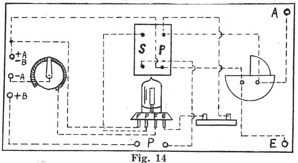
lected. Do not forget that where there is a semi-circle at wire crossings the wire must be kept well apart. The valve in this case, too, may be "cushioned" on its connecting wire behind the peep hole. This peep hole can be left out if so desired.
