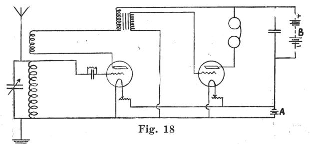
of the amplifier is IS; that from the positive of the "B" battery to IP; and that from the negative of the "A" battery to OS. The loud speaker is connected in place of the telephones.
