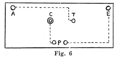
carried out at the back. The letters on Fig. 6 represent: "A," aerial terminal; "E," earth terminal; "T," catwhisker terminal; "C," crystal cup; "P," phone terminals.
