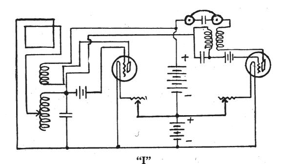
**Circuit I.**—Is a simple two valve super-regenerative circuit. The "hook up" is shown here with a loop aerial. The primary and secondary should have values to suit the desired wavelengths and be so arranged that they can be tightly coupled. The other inductances are for the purpose of producing suitable frequencies in the oscillator valve circuit. The frequencies should be so arranged by means of the condenser (.0025 mf) in this circuit that they are just above audible frequency.
