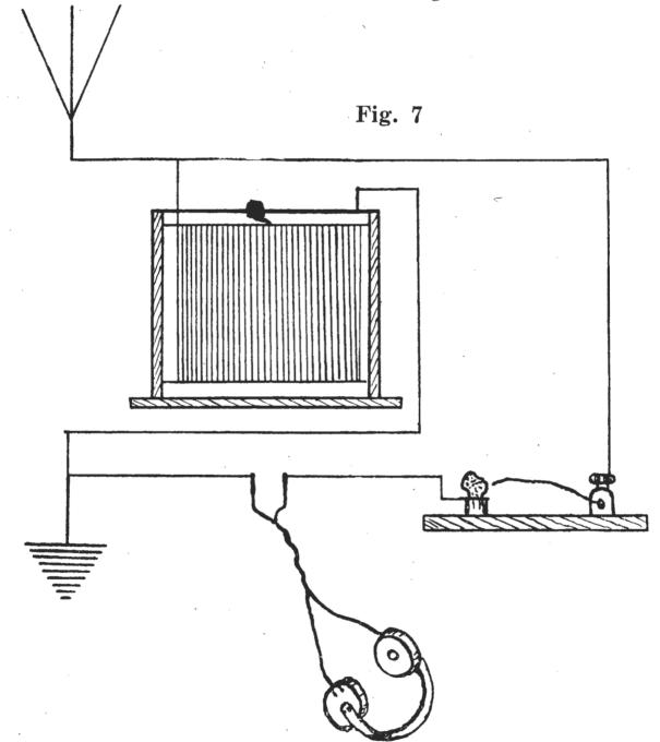
the slider slowly along till signals are heard. Then try various parts of the crystal for the most sensitive spots where the signals come in loudest.
