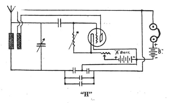
**Circuit H.**—This is the famous Flewelling hook up. It is a superregenerative circuit and when properly constructed and well operated will give splendid results. But the circuit is a difficult one to handle.
