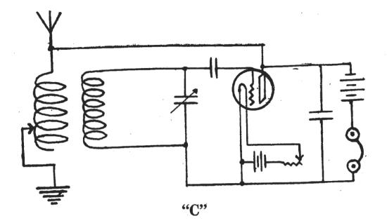
**Circuit C.**—In this circuit a feed-back effect is obtained by connecting the plate to the aerial. This circuit is not particularly good for telephony work as it is not easy to control the oscillations.
