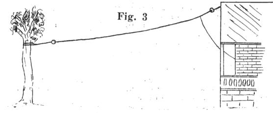
to the set, and should be kept as short as possible. The portion of wire cut from the aerial should be used for the "lead in," and care should be taken to attach it properly to the aerial. It is necessary to do more than just twist the wire round; it should be soldered.
