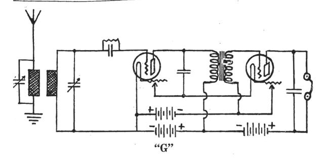
**Circuit G.**—This circuit has been designed for two valves, detector, and audio-frequency amplifier. Honeycomb coils are used. The fixed condensers shunting the 'phones, and primary of the transformer should have a capacity of .001 mf. Properly wired up and using a suitable inter-valve transformer (one, the curve of which is comparatively flat over the 100 to 5000 cycles per second range), the circuit will give good results on broadcast reception.
