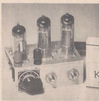
though the circuit arrangement (Fig. 4) is similar to the 15-watt version, a few minor modifications have been made. The amplifier is capable of excellent reproduction with less than 0.3% distortion and has chassis dimensions of only 3 x 4 x 13 inches. From this. with a suitable power supply, a virtually - dis-
