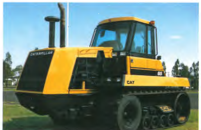
Caterpillar tractor employing rubber tracks.
