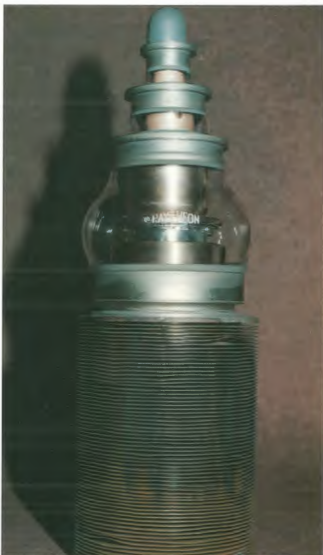
Matchless ML6427 valve with horizontal cooling fins employed in VLW 50 kW transmitter STC type 4-SU-61.
