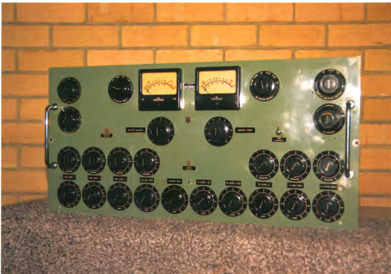
Mixer unit used in 1960's for AM stereo broadcasts and recordings.
