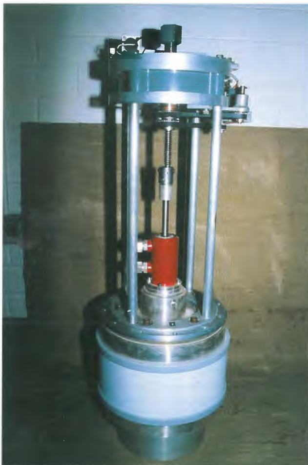
Modified Comet capacitor ready for fitting into the transmitter.
