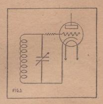
Resistance method of eliminating oscillation.
