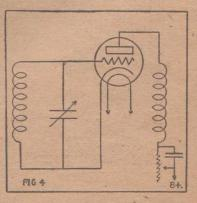
By varying the plate voltage of a valve oscillation is controlled.
