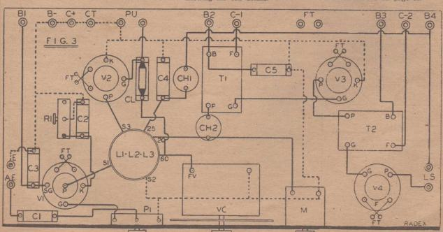
Layout of the components for the four valve receiver.
