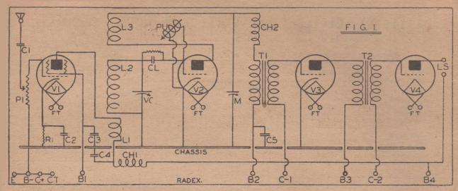
Schematical diagram of the Quality four valve receiver.
