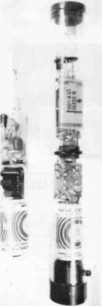
Two versions of the Flasher. On the left, one from a junked photo flashgun; on the right, from overthe-counter parts.
