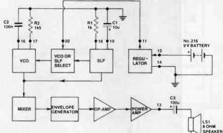
Above: Circuit for the ETI-607C Alarm. It produces a 'woopwoop' sound. Overlay is at right.
