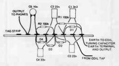
As with the simple crystal set, we mounted the components for the voltage-multiplier crystal set on an eight-lug tag strip. We have supplied a drawing as it is clearer than a photo in this instance.
