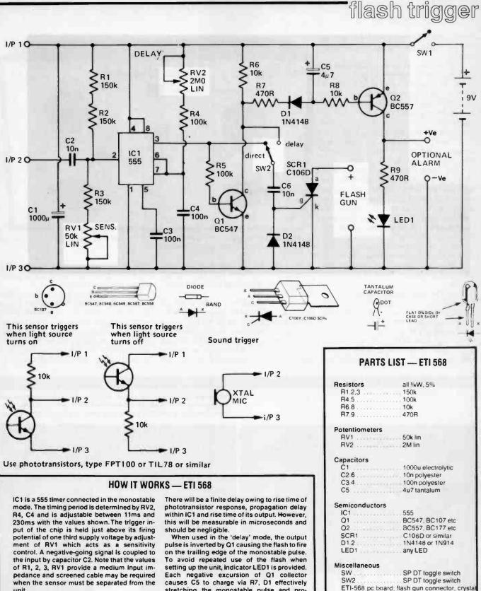
When IC1 is 'fired' its output (pin 3) goes high for the monostable period. With SW1 switched to 'direct', this positive going pulse will fire the SCR and discharge the flash enabling the unit to be used as a slave flash.
