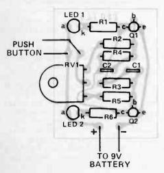
Fig. 2. Layout of the printed-circuit board version.
