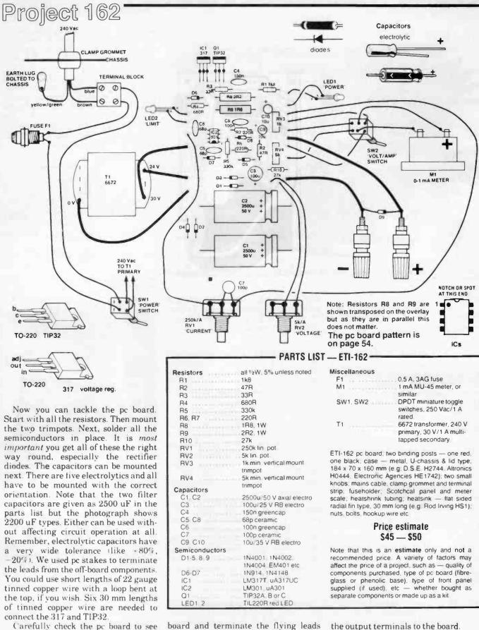
Carefully check the pc board to see that all components are mounted and the semiconductors and electrolytics are correctly polarised. Mount the pc 58 the output terminals to the board. All OK? Check it!
