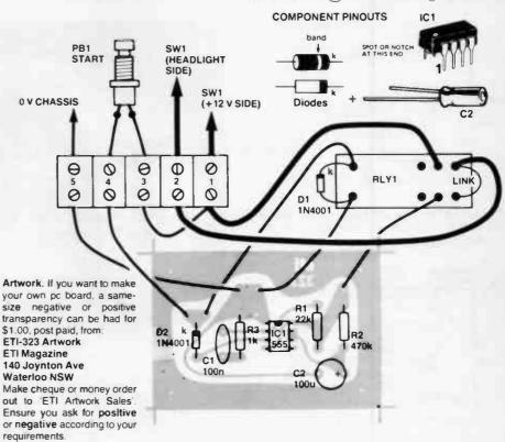
**Component overlay and external wiring.** How the parts are assembled onto the printed circuit board — watch which way around you assemble D2, IC1 and C2. Wiring to the external components is also shown. The pc board and relay may be housed in any suitable box, if you wish.
