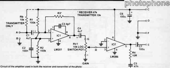
Circuit of the amplifier used in both the receiver and transmitter of the photophone. Note that Rb is used only in the transmitter and that the value of R3 differs between the transmitter and receiver.
