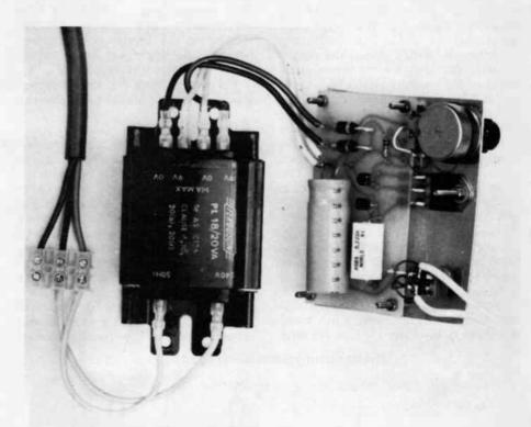
within this specification are the requirements that the mains input connections be shielded, that they be on the opposite side of the transformer from the output, that specially heavy insulation be used (in that the primary winding is kept right away from the secondary winding) – and so on.
