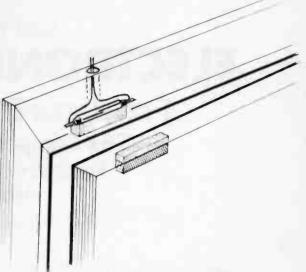
Door protection -- the reed switch is set into the architrave.
