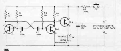
via R1 and the base of Q2, keeping Q2 on while it charges. C1 will begin to charge via R2, and when the base voltage on Q1 has risen sufficiently, Q1 will commence to conduct. The collector voltage on Q1 will rapidly fall. This will cause the charge on C2 to reverse-bias the base of Q2, immediately turning it off. Thus, the collector voltage on Q2 will jump to the supply voltage and C1 will begin to charge via R4 and the base of Q1, holding it on while C1 charges.
