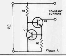
about 0.5 - 0.6 V, Q1 will turn on. Current through R1 will then be shared between the base of Q2 and the collector of Q1.
