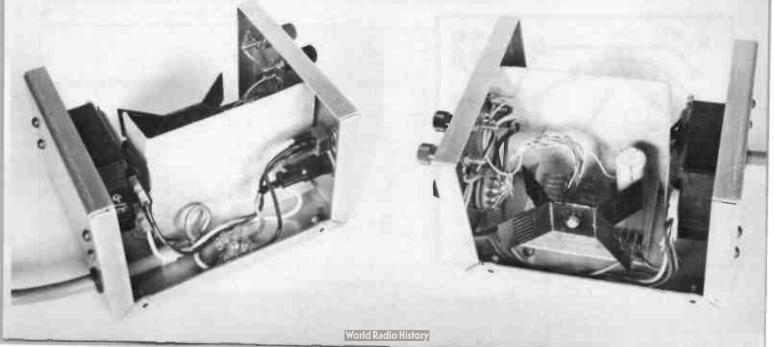
component. Check that adequate clearance is allowed for later wiring and access.
