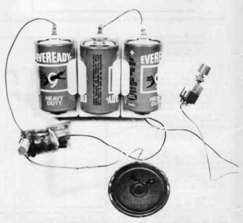
A small loudspeaker serves as both microphone and speaker in this intercom. Housing the project we have left up to you. It is quite possible to fit the components in a palm-sized box, such as one of the small 'zippy' boxes available inexpensively from a number of suppliers. The intercom may be powered from a 3 Vdc plugpack if you wish.
