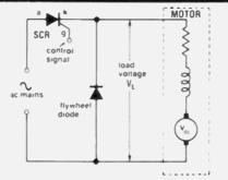
Figure 2. Fundamental circuit elements of the controller used in this project. Note that  $\left|V_{dc}\right|$  is the back-emf of the motor.
