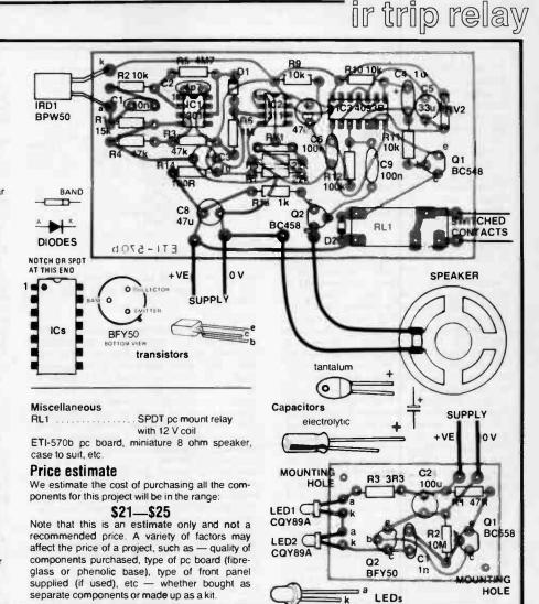
as our layout diagrams show, and take care when soldering them in that you don't overheat them. Use a reasonably small bit, don't spend too long over each pin and allow the whole IC to cool down for a few seconds between soldering each of the pins.
