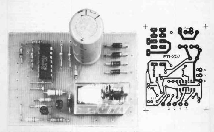
The relay driver board is simple, yet versatile. The external input/output pins are located around the edges of the board.
