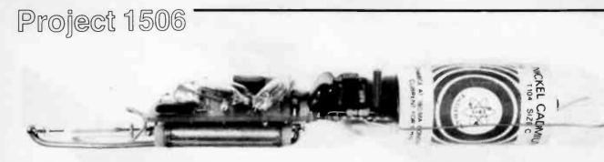
Overall view of the Flasher constructed from a cannibalised flashgun.
