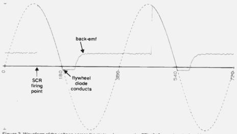
Figure 3. Waveform of the voltage across the motor when using the ETI-1515 speed controller (Vertical axis not to scale.) The dashed line shows the mains input waveform
