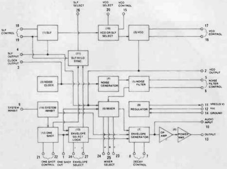
Internal block diagram of the SN76488.
