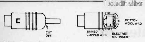
Making the microphone. A DIN plug is modified as shown to house the electret mic insert.
