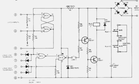
Circuit diagram of the relay driver board. Note that the rectifier diodes may be any of a range of types, such as 1N4001-2-4, etc, or EM401, EM402, etc. A variety of common relays will fit the pc board.
