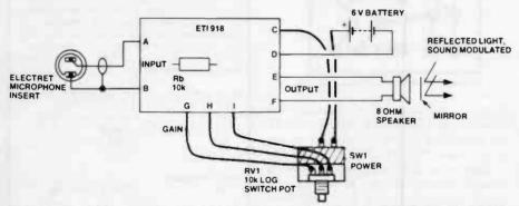
Wiring diagram of the photophone transmitter. Note the wiring to the rear of the electret microphone insert. You'll find one connection attaches to the mic case. This is the 'common' and goes to B on the pc board. Some inserts have leads already attached. Usually the common lead will be black. Use a shielded lead between the mic and the input to the amp.
