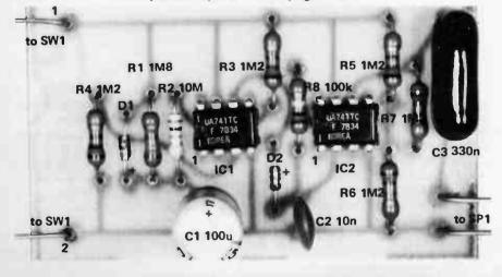
the plate or hard as nails) the timing resistor R1 can be substituted with a 2M or 5M trim pot, or could even be a potentiometer mounted on the front of the box. As the circuit draws no current when it is not being used it should give very good battery life, unless you forget to switch it off (but boy, is that noise annoying after five minutes!).
