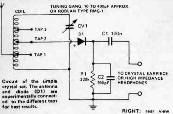
from the diode to earth 'shorts out' or 'bypasses' the RF signal, leaving the audio which is then fed to the earpiece.
