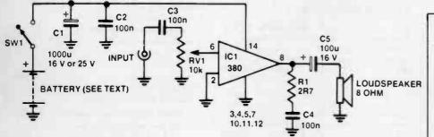
mount on the non-copper side of the board. Next identify the positive and negative leads of the two electrolytic capacitors. These are 'polarised' devices and can only go in one way. Solder them in place, putting the positive lead of each in the hole marked with a '+' on the overlay diagram.
