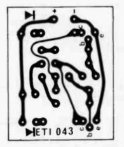
Fig. 4. Printed circuit board layout – full size 40 x 50 mm.
