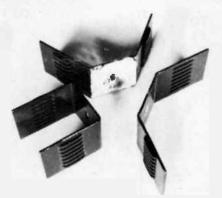
The heatsink we used for Q2 was made up from two 'flatpack' heatsinks, Dick Smith No. H3402, bent as illustrated and mounted back-to-back on the transistor. This ensures they fit in the case. Use plenty of silicone heatsink compound to get good thermal conduction. The unmodified heatsink is shown at lower left.
