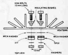
Mounting the 317 regulator and TIP32 transistor to the heatsink.
