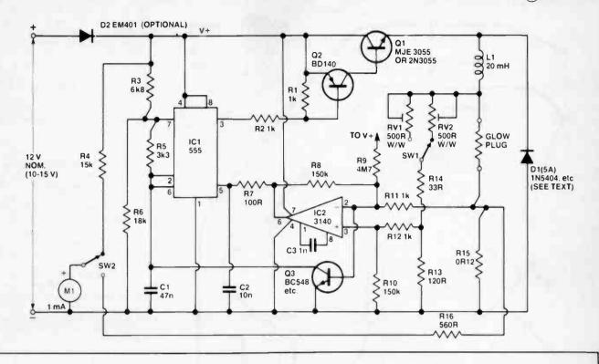
$({\rm I}_{\rm L})$  flows, is sensed by Q3 which provides current-limiting.
