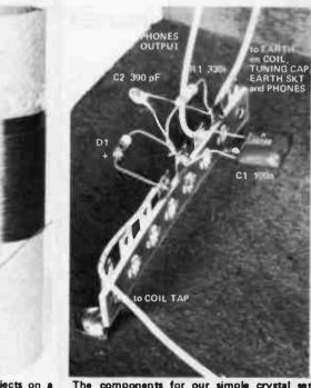
We wound the coil for these projects on a former cut from a cardboard mailing tube. The matchstick is slid under each of the turns to be tapped. Clean the enamel from the wire at each tap to get a good connection.
