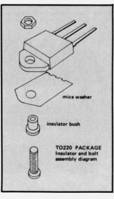
as shown in the photo of the prototype. The cases of these transistors are connected to the collectors and must therefore be insulated from the diecast lid. Mount the transistors using a mica or plastic insulator and plastic sleeves as shown in the diagram. Use an ohmmeter to check that there is an open circuit between the collectors and the diecast lid after the transistors are mounted.
