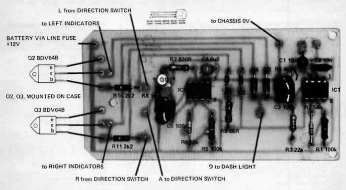
Component overlay and external component connections.
