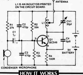
This circuit is basically an oscillator which runs at around 100 MHz. The most important parts of the oscillator are the transistor Q1 and the tuned circuit, which comprises the inductor L1 and the variable capacitor CV1.
