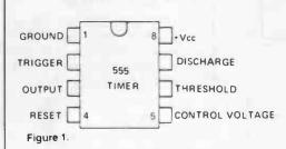
The 555 timer is a very versatile IC designed specifically for precision timing applications
