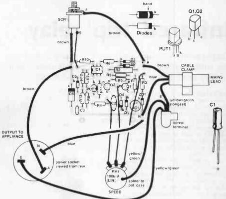
Overlay and wiring diagram. Follow this to assemble the pc board and wiring up of the external components. The pc board pattern is on page 90.
