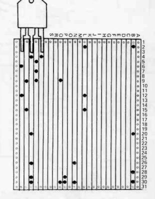
Veroboard solder connections – note no break holes are required in this board.
