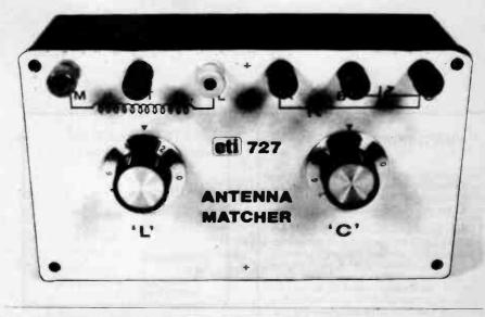
The project is housed in a plastic utility box, the front panel being dressed up with a Scotchcal Panel.
