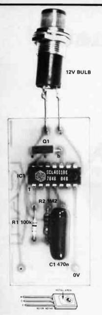
To turn a lamp on and off requires a little more circuitry. We couldn't connect the lamp at the output of IC1b as it would rapidly discharge C1 at the wrong time! To switch the 150-200 mA required by the lamp, we use a transistor to amplify a small current supplied to its base, the lamp being connected between the emitter and the negative side of the supply. This sort of circuit is called an "emitter follower". This is a current amplifier.
