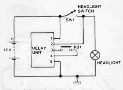
Figure 3. Connection of the delay unit to a car system where the headlights are independent of the ignition switch
