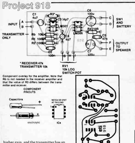
higher gain, and the transmitter has an extra resistor (Rb) to bias the microphone. Only a small speaker is necessary for the receiver, so that a nine volt transistor radio battery can be used as power source.
