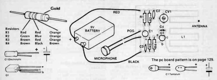
disconnect the battery when you're not using the unit. Of course you can insert a switch in one of the battery leads if you prefer.
