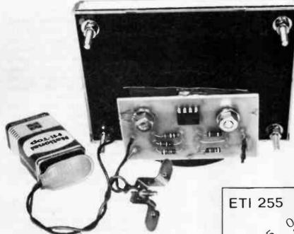
Rear view of the instrument showing general assembly. You may prefer to use a rechargeable NiCad type, rather than the dry battery shown, for battery operation of the unit.
