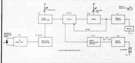
continuous series of pulses from the transmitter keeps C3 discharged, with a low voltage across its plates. If the beam from the transmitter is interrupted, C3 charges up and the voltage across it rises.
