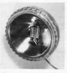
Close up of our receiver input device. This consists of a small solar cell piece mounted in a reflector taken from a 'Dolphin' lantern. To mount the cell, we cut a slot in one side of the reflector, put Silastic on the rear of the solar cell (leads already attached) and inserted it in place. It proved very effective.
