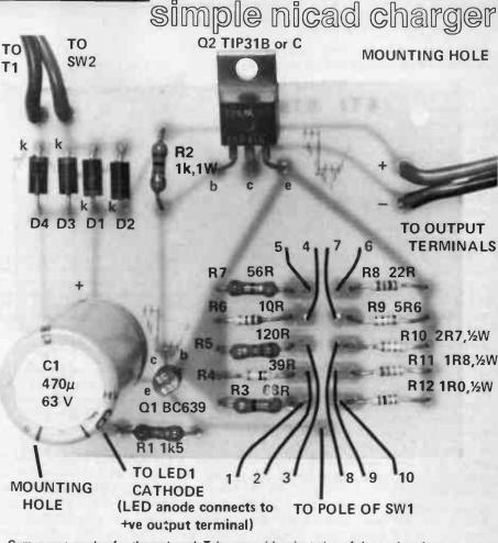
Component overlay for the pc board. Take care with orientation of the semiconductors.
