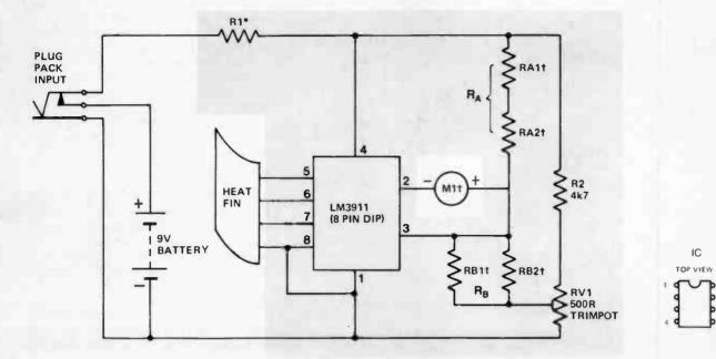
\*R1 = 470R ( $\frac{1}{2}$ W or  $\frac{1}{2}$ W) for 9 V operation; 1k8 for 12 V battery (11 - 15 V) operation. †See table below for resistor values to suit different meter ratings.
