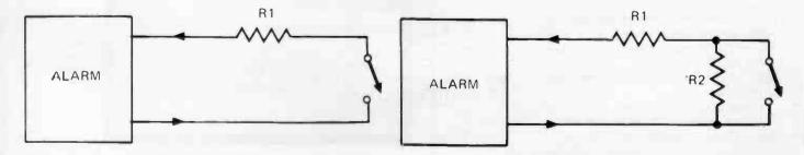
Figure 2. Resistance R1 represents series resistance of the loop (see text). Resistance R2 represents leakage paths across alarm contacts.
