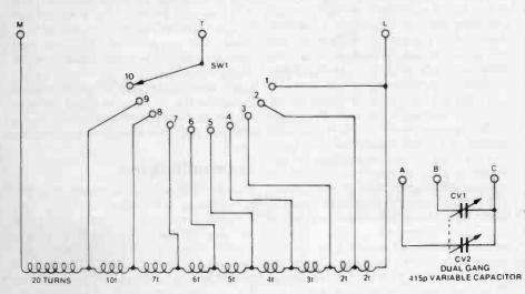
General circuit diagram, showing the number of turns on each coil section.
