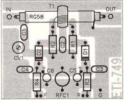
The component overlay for the ETI-749 SWR Meter. This was shown incorrectly in the January issue, on page 124.
