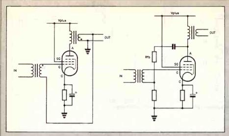
Figure 9.7. Two ways of applying negative feedback to a power amplifier.
