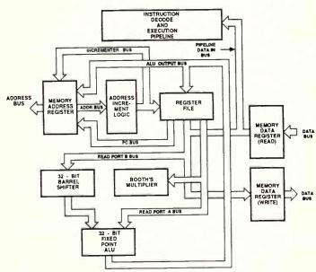
Figure 5. Internal block diagram of the VL86C010 RISC processor.
