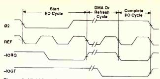
Figure 8. VL86C410 Interruptible cycle example.
