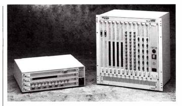
products and provides a sophisticated backplane designed to support multiple access methods such as Token Ring and Ethernet.
