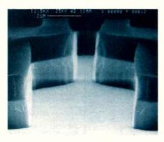
GaAs feature etched in a chlorine based ECR plasma using a 1.5  $\mu$  m positive result mask.
