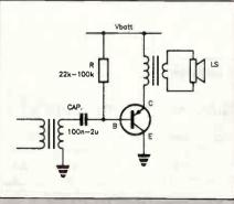
Figure 9.9. A typical single transistor power amplifier.
