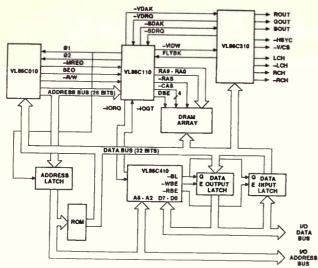
Figure 1. Block diagram of a RISC system based on the VL86C010 Acorn RISC Machine (ARM) and its companion support chips.
