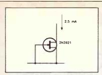
Figure 9.14. Simple form of FET current source.
