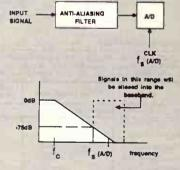
Since the filter loss is greater than 76 dB, any alased signals will be below the 12 bit level.
