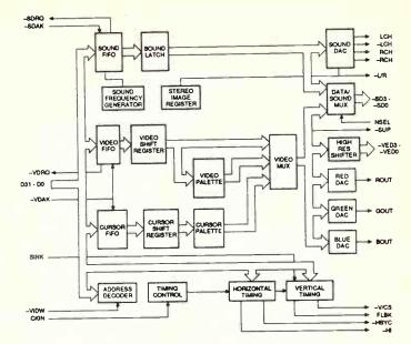
Figure 6. VL86C310 video controller (VIDC) block diagram.
