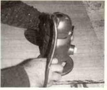
Chamfer the driver cutouts with a router if you mount the drivers behind the front panel, as I did.
