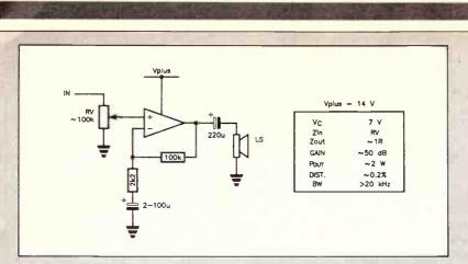
Figure 9.10. Single IC power amplifier. Not much to it!
