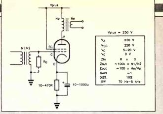
Figure 9.6. Single beam tetrode transformer coupled power amplifier.
