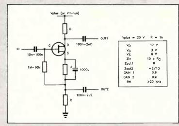
Figure 9.4. An ac coupled FET phase splitter.
