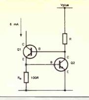
Figure 9.15. Two-transistor accurate constant current source. You'll see this widely used in many applications.
