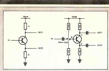
Figure 9.3 Single transistor dc and ac coupled phase splitters.
