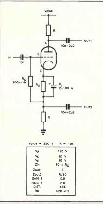
Figure 9.2. An ac coupled phase splitter.
