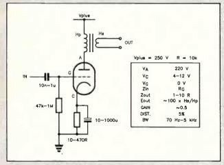
Figure 9.5. Single triode RC coupled AF power amplifier.
