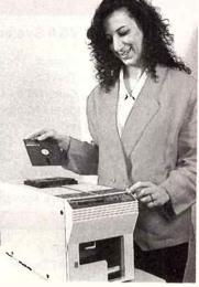
previously made copies and quickly formats blank diskettes. The internal 30Mb hard disk drive stores master images for both 3.5-inch and 5.25-inch applications.
