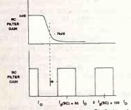
Note: The RC filter should provide > 76 dB of loss to several different SC filter sample rates  $f_{\rm S}$  (SC).
