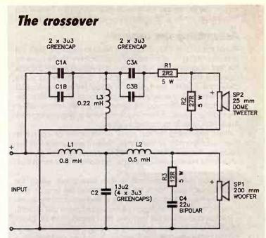
Circuit of the crossover. It's a 3rd-order (18 dB/octave slope) type, with the crossover point set at around 2.5 kHz.
