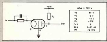
Figure 9.8. A grounded grid power amplifier.
