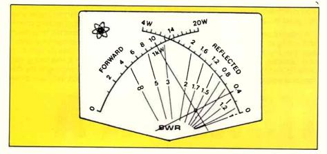
How the cross needle display works. The dual meter movement indicates forward power on the left hand scale and reflected power on the right hand scale. Where the meter needles cross shows the SWR according to the vertical line markings (they're arcs, actually).
