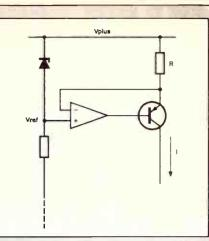
Figure 9.16. IC-transistor constant current source.
