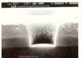
Features etched in silicon dioxide by ECR method. Processes previously requiring side wall polymerisation can now be done under polymer free conditions, thus eliminating particle and residue problems.
