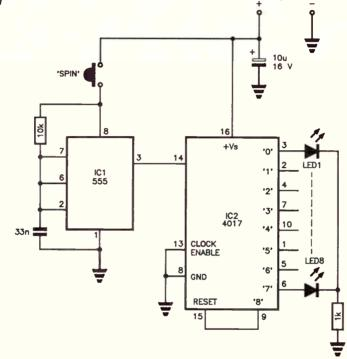
when you release the spin button, stopping the 555. You can observe the action of the lights "going round and round" if
