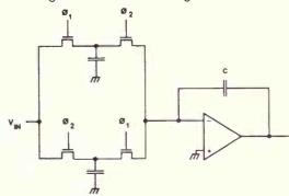
Figure 4. SC double sampling input.
