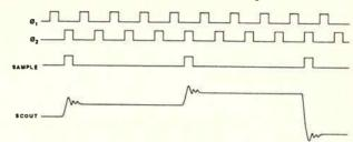
Figure 7. S/H sampled SC filter output.
