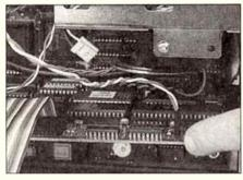
One flying lead you may not have been able to connect, depending on whether or not you have a hard disk, is the connection for the hard disk operation indicator. This attaches to the hard disk controller card and so can only be connected once this is installed.
