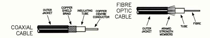
Illustrating the differences between the construction of coaxial cable and today's fibre optic cable.
