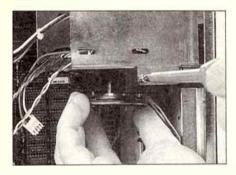
The speaker and its mounting hardware are then secured, using a self tapping screw, to the plate of metal protruding from the underside of the drive enclosure inside the case.
