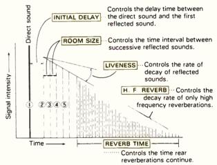
By changing the parameters of a preset program, you can create different sound fields. The six parameters are: 1) Initial delay; 2) Room size; 3) Liveness; 4) Reverb time; 5) HF reverb and 6) P front EQ, rear EQ.
