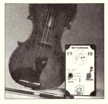
The metronome needs a loudspeaker output giving sufficient volume to be heard above the instrument, or instruments, and for convenience, it must be portable. This means battery operation, ruling out powering it from the mains.
