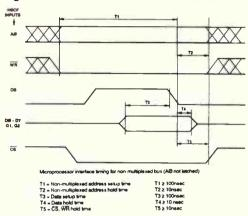
Figure 12. Timing diagram for non-multiplexed bus.
