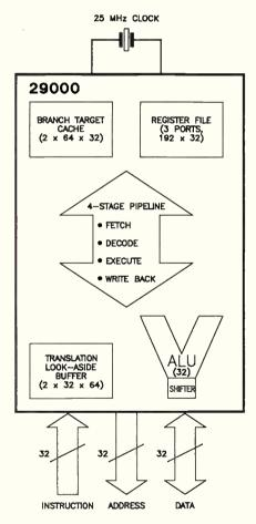
Figure 2. AMD's 29000. Note the 4-stage pipeline and large register file, features you'll see in other RISC processors.
