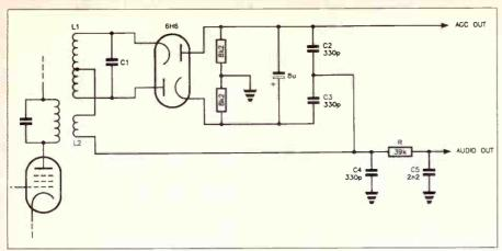
Figure 8.9. FM ratio detector.
