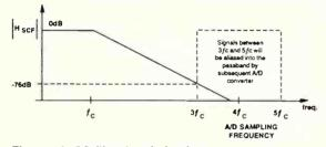
Figure 16. SC filter bandedge loss.
