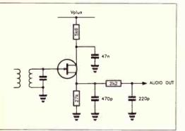
Figure 8.7. FET infinite impedance AM detector.
