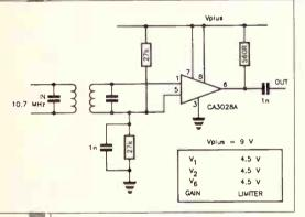
Figure 8.3. IC RF/IF limiting amplifier.
