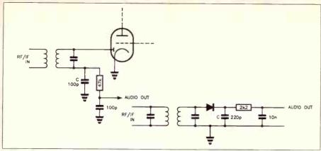
Figure 8.5. Diode AM detectors.
