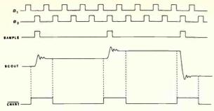
Figure 8. CNVRT\ timing.
