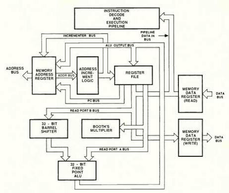
Figure 5. Block diagram of the VLSI VL86C010, a low cost RISC processor.
