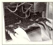
Re-installing the add-on cards is the next step, after checking all flying leads are properly connected. This is a simple matter of sliding the card into an appropriate slot and 'rocking' the card slightly in order to secure it in the edge connector on the motherboard. Be careful not to put too much pressure on the motherboard as it may flex the board to a point where it cracks, or breaks a track.
