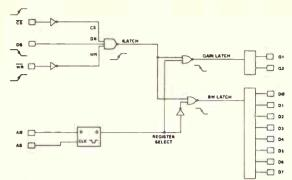
Figure 10. Equivalent latch logic.
