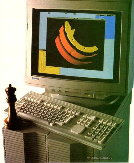
The Tektronix XD88 graphics superworkstation is a high performance unit based on the Motorola 88000 RISC processor.
