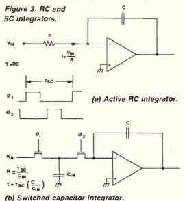
two-phase, non-overlapping clocks: Ø1 and Ø2. The period of these clock signals is  $T_{\rm SC}$
