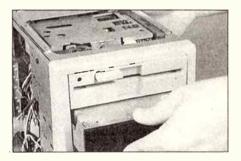
The hard disk is installed in the same manner as the floppy drives. However, only hold it by the front panel and the rear skirt on the chassis. Don't let your fingers stray into "the works".
