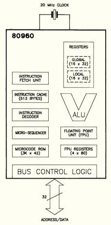
Figure 1. Architecture — or block diagram — of Intel's 80960 RISC processor. Bit of a mix of RISC, CISC and microcontroller.
