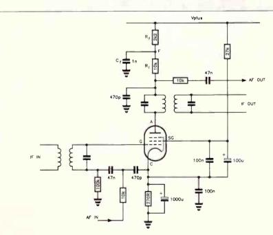
Figure 8.4. Reflex amplifier that amplifies both IF and AF voltages.
