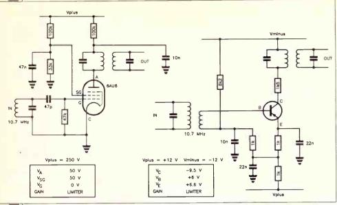
Figure 8.1. Valve RF/IF limiting amplifier.
