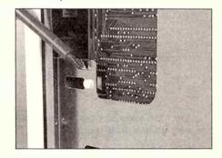
As can be seen in the picture the case provides for the mounting of the main computer board using copper and nylon
