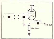
Figure 8.6. Valve infinite Impedance AM detector.
