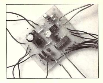
important; get one or more wrong and it won't work, apart from the possibility of damaging an IC, for instance. Note that the 4017 (IC2) is a CMOS type and, while it features protected inputs, follow the usual precautions for handling CMOS: only pick it up by the ends and avoid touching the pins. Solder its ground (pin 8) and supply (pin 16) pins before the others.
