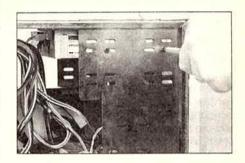
Once the drive is in position, four screws are needed to secure the drive to the case. I have noticed in doing the three different installations that the types of screws needed to do this vary from drive to drive. If there are no suitable screws in the hardware supplied with the new case you should use the screws left over from your old system.
