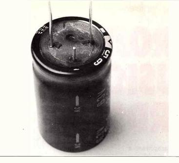
Most RB-type capacitors have a third lead, which is the very short lead you see in this photograph. This lead is used to properly locate or orientate the component, as well as provide some mechanical stability when soldered to the pc board.
