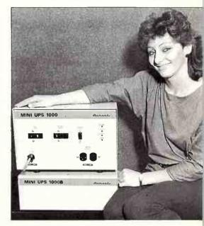
The ultimate protection is provided by an uninterruptible power supply, or UPS. Shown here are two models of a 1000 VA UPS from Densei.
