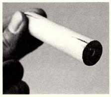
The wooden dowel is prepared by drilling pilot holes in each end for the eye hooks and cutting a slit down each end to pass the balun's connections out to the antenna feedpoint.
