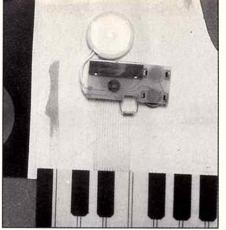
A mini-piano module revealed! The keyboard connecting strip can be clearly seen, the metal strip at the top of the board clamps it in place so that it contacts with tracks on the pc board. The resistor is referred to in the diagrams and text here as 'Rosc'.
