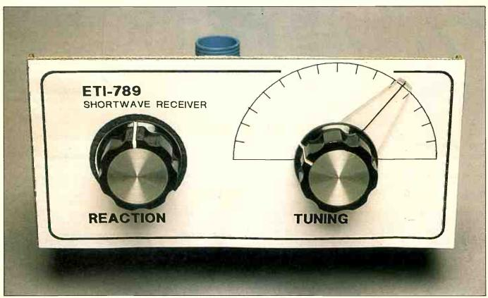
Front view of the completed project. The cabinet is made from pieces of blank board soldered together and measures 168 mm x wide 80 mm high x 108 mm deep.
