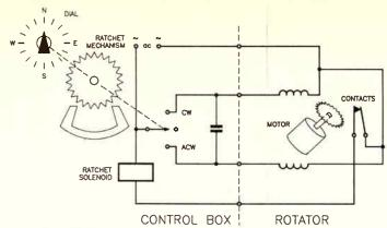
Figure 4: simplified schematic of the simplest, lowest-cost style of control/indicator unit, employing a ratchet-and-solenoid escapement mechanism. Light duty "TV-type" antenna rotators have control/indicator units of this type.
