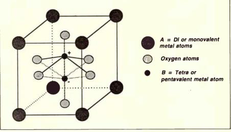
Figure 1: simplified ferroelectric molecule type ABO<sub>3</sub>.
