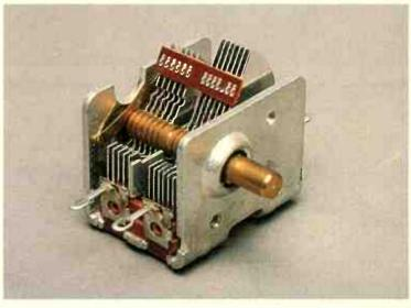
Picture of a two-section tuning gang of the type that can be commonly salvaged from an old radio or found in some suppliers' stocks. Only one section is used, the one with the larger set of moving plates. This provides a wider tuning range. Use the other section if you want a lesser tuning range.
