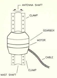
Figure 1: the shaft-mount or coaxial style of antenna rotator. Light duty "TVtype" rotators are like this.
