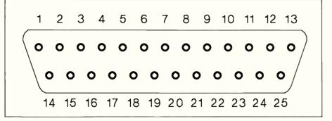
The 25-pin D connector arrangement, looking at the pins of a plug or the connections (rear) of a socket.
