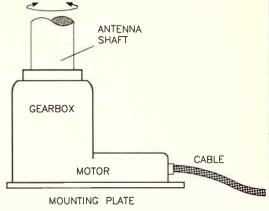
Figure 2: this type of rotator is designed for mounting on a plate and incorporates a thrust bearing and motor in the base. Medium and heavy duty rotators are of this type and may incorporate an antenna shaft mounting arrangement rather like the coaxial type shown in Figure 1.
