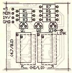
Overlay, showing the component positions. Note that Q1, R1 and R2 are optional. Note also the two possible positions for the LT313 7-segment displays. The solid lines indicate the placement for a "4.7/8.0" display, the broken lines indicate the placement for a "HI/LO" display.
