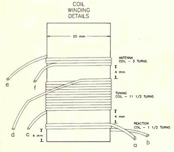
Figure 2: coil winding details. Use 20 gauge enamelled copper wire. All turns are wound next to one another (closewound).
