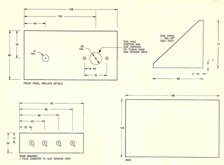
Mechanical details of the cabinet, which is made from pieces of single-sided pc board. All dimensions are in millimetres.
