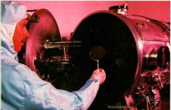
ABOVE: Ramtron's proprietary process involves adding a layer of ferroelectronic lead-zirconate-titanate (PZT) to the existing semiconductor underlayers. LEFT: In Ramtron's class 100 clean room facility, standard semiconductor development and fabrication techniques are used to incorporate ferroelectronic materials onto silicon wafers.
