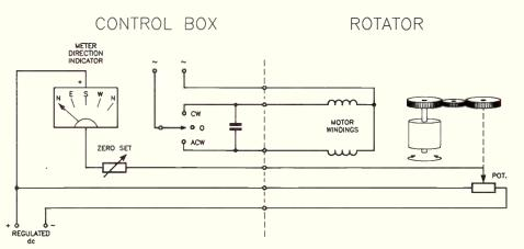
Figure 5: this style of control indicator/unit is popular, found on mid-priced medium duty rotators. A panel meter serves as the indicator.
