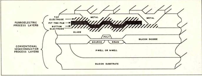
Figure 2: PZT thin film on CMOS.
