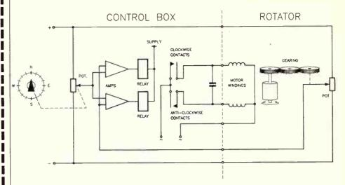
Figure 6: the more sophisticated style of control/indicator unit has a schematic rather like this, known as a balance-type circuit. Heavy duty and some medium duty rotators sport control/indicator units of this type.
