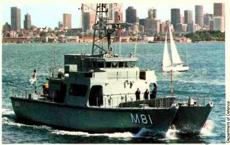
HMAS Shoalwater, now fitted with bilge keels, has put hull problems behind it, says the navy.
