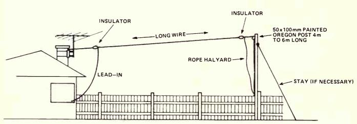
Figure 3: a useful long wire antenna for your shortwave receiver. You can use hookup wire, for economy. The insulators can be egg insulators obtainable at electronics stores.
