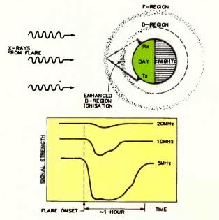
Figure 5. How X-rays from a flare affect HF signals, causing a shortwave fadeout on the dayside ionosphere. Note how the lower frequencies are affected most. The X-rays cause a sudden, large increase in ionisation in the ionosphere's D-layer, which increases absorption of the signals.
