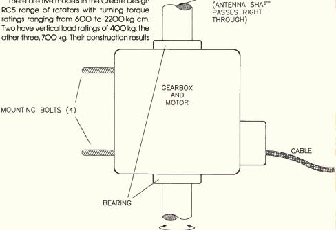
Figure 3: this through-shaft type of rotator is less common than the other two, more often seen as an elevation rotator, for satellite antenna systems. The antenna shaft passes right through the gearbox and motor housing, with shaft clamping arrangements adjacent to the bearings at each end.
