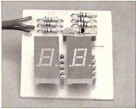
View of the completed display board. From this you can see how the LT313 7-segment displays are oriented. Note that this prototype requires an inverted input (explained in the text).
