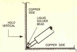
Figure 1: once the cabinet pieces are tacked together, a fillet of solder is run along each of the mating edges as shown here, making sure the iron tip heats both edges such that the tinning you put on initially liquifies. Touch the solder to the iron tip where it meets the two faces so that a liquid solder bead forms, then slowly run the iron along the joint.
