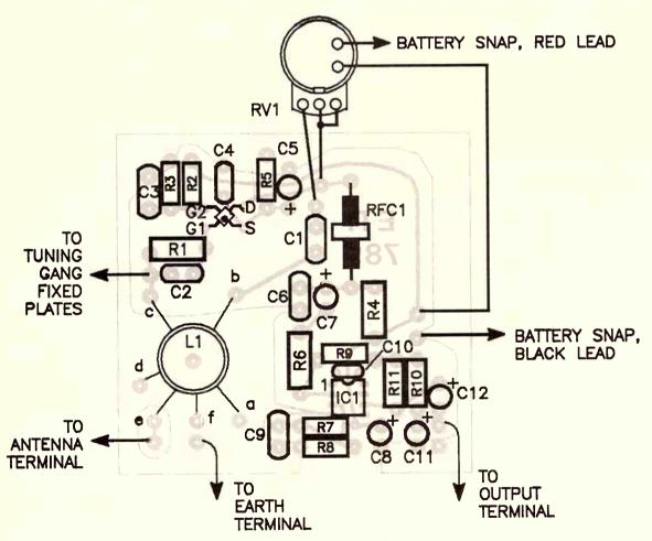
Component overlay for the printed circuit, showing where the various components are placed and the off-board connections. You can complete the wiring to the off-board components by reference to our "inside" picture of the project.
