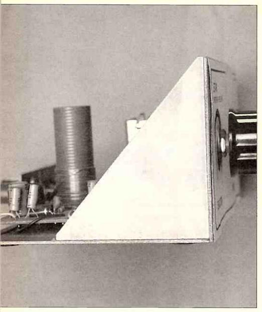
Side-on view of the cabinet, showing how the cabinet pieces mate together.
