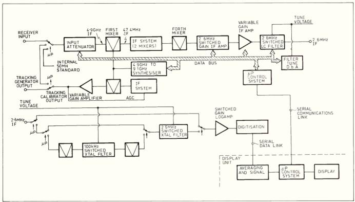
Figure 1: Block diagram of the Marconi 2383.
