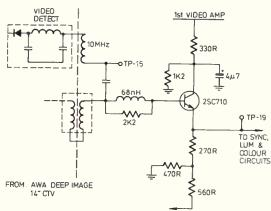
A TV is unlikely to give true high resolution comparable to a monitor but by injecting a video signal to the video stage of a TV, the improvements can be substantial. The reason is simple and twofold. A computer to TV
