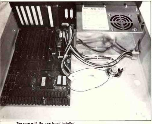
The case with the new board installed.
