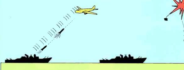
Figure 3: SPY 1 steers missile radar onto the target. When the missile radar acquires the Airbus, the SAM is launched. Aegis computer guides the missile towards the target.
