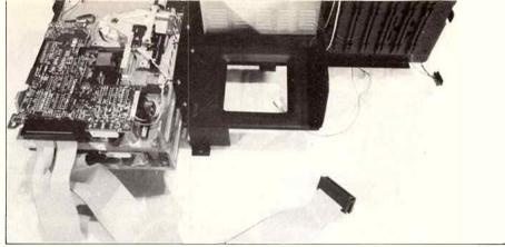
A close up of the front panel with all the disc drives, which comes away as a complete unit. Removing this makes access to the board very simple.
