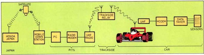
Honda powered McLaren Formula I rocing cars have a potent communications link behind them, so that engineers in Japan can study the car's performance in detail, no matter where it is racing.
