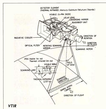
The Visible and Thermal Infrared Radiometer covers one visible and three infrared bands to detect thermal radiation for the earths surface. This instrument is equipped with a rotating scanning mirror which mechanically scans the earth's surface from right to left. Things are arranged so that the mirror is either looking at the earth's surface, an
