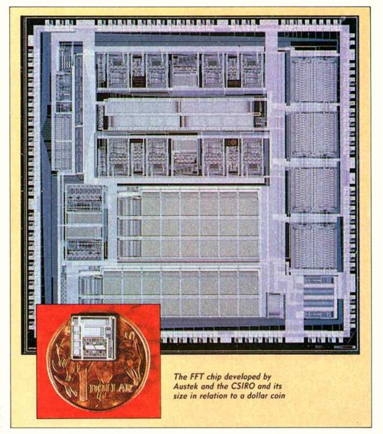
junction with Austek Microsystems. The chip performs FFTs on digital data in real-time. It has been quoted that the prototype chip performs a FFT process a hundred times faster than a \$150,000 Vax computer. In the past FFT algorithms have been implemented in software using either general-purpose signal
