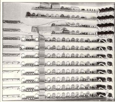
The underside of the mixer, All connections to the boards are made via the ribbon cable.
