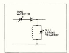
Figure 2: Generalised adjustable filter
