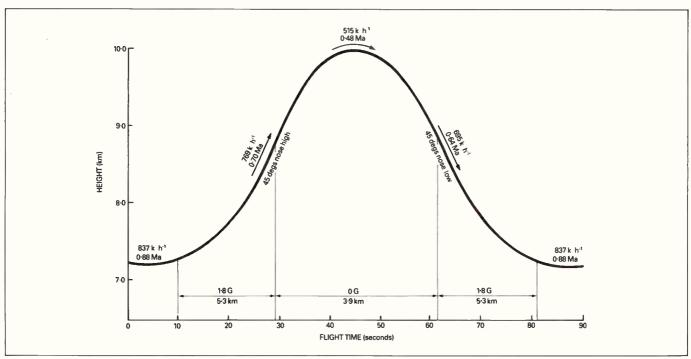
Profile of a typical parabola flown by NASA's KC135 aircraft.
