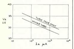
Figure 2. — Iso-Exposure Graphs for a Typical Cathode Ray Tube
