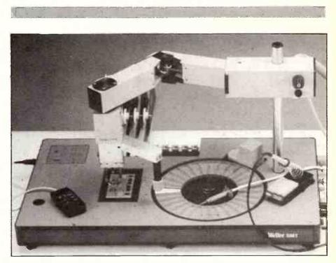
The Weller PPS is one of a new generation of manually-controlled machines designed for working with low volumes of surface-mount products. In fact it is ideal for prototypes and repair work. The carousel at right holds all the components. At left is a vacuum lifter to pick up the components, and a heater to melt the solder. Courtesy Cooper Tools.
