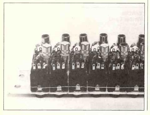
merely involves making the 'patch' with a short lead. A sophistication of this basic idea is to have commonly connected items (such as the stereo output of a mixer and the mixdown recorder) *normalled* via the patch bay so that unless a patch lead is plugged in the connection is automatically made to the desired piece of equipment. Specifications:
