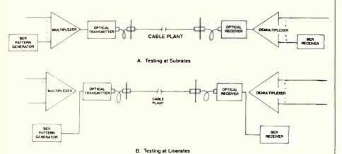
Figure 9 Bit Error-Rate Measurements
