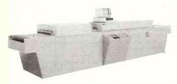
A typical modern reflow soldering system from Vitronics. It is intended as an integral part of the manufacturing line of the future - the boards go in one end, the operator does a bit of programming in the middle, and the finished boards come out the other. The messy, smelly, dirty process of wave soldering can at last be consigned to the bin. Courtesy Penn Central.
