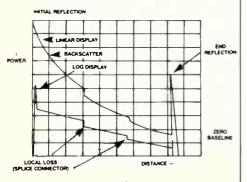
Figure 5 Typical OTDR Display
