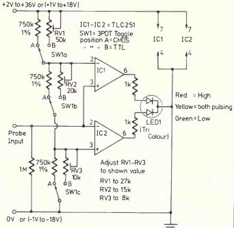
enough, between high and low states, the two LEDs will appear permanently lit, resulting in a yellow colour. Static voltages are not shown by LEDs, but are indicated by no LEDs on. With no input but voltage applied to the circuit, the green LED will be on.
