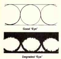
Figure 12 Examples of Eye Diagrams
