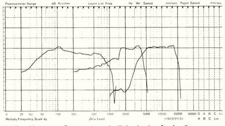
The effect of the crossover. The traces were made with the microphone 5 cm from the woofer, mid-range and tweeter to show the performance of individual drivers. Vertical scale is in dBs and horizontal in Hz. Concerto No. 1 and Rachmaninov Piano Concerto No. 2, Decca 421181-2. I could shut my eyes and imagine myself in the front row of the Opera House without any trouble (and as I did not have to go — far less trouble). Once again the Dali 40s really shone.
