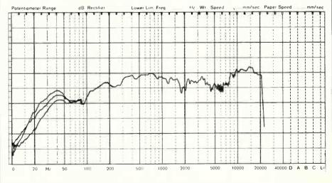
Three frequency response traces showing the effect of the LF response plugs.
