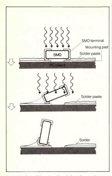
Tombstoning is one of the major problems facing surface mount manufacturing. If the solder does not melt on both pads simultaneously then the surface tension of the solder mass that first melts will pull the SMC upright. This can be caused by insufficient metalisation of the component itself, uneven wetting of the terminals, asymmetrical pads or different amounts of solder on the pads. Courtesy Siemens.
