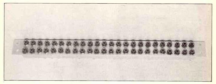
switch on its respective socket) then the connection is said to be normalled, ie, with no plugs plugged into those sockets the signal will be sent from FX1 to the input of the reverb unit.
