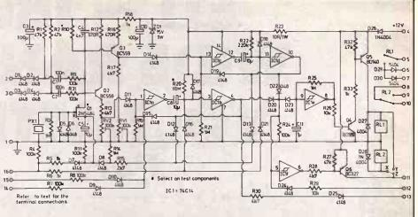
turn on transistor Q6 via resistor R28. Transistor Q6 will in turn supply nearly full supply voltage at terminal 11 and if the link from X to Z is connected relay RL2 will be activated.
