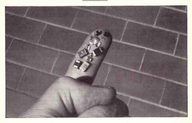
Surface Mount Devices (SMDs) are likely to have replaced at least 50 percent of conventional, leaded components (components which have leads) on new printed circuit board assemblies by 1990, according to the giant electronics company Siemens.
