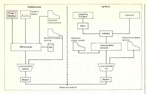
Remote operations network for the optical telescope sited at La Palma.
