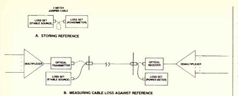
Figure 4 Loss Measurements on Cable
