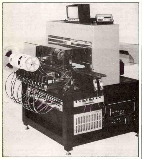
A typical 'entry level', (ie: cheap) surface-mounting machine is this Omniplace 4618 from Universal. It can place components to an accuracy better than 0.025 mm. The components enter the machine mounted on the bandoliers at left. The boards enter at right. The machine is fully programmable and comes with a controller with 256K of memory on board. Courtesy Universal.
