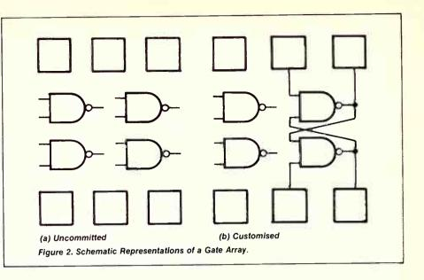
routing channels surrounded by buffers configurable as either input or output. Figure 2 (b) illustrates a completed gate array customised by a single metal interconnection layer defining its function as a simple latch. In a gate array the percentage of active area is typically 25 per cent, with the remaining silicon allocated to wiring space.
