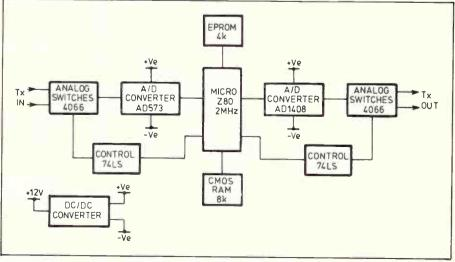
Figure 2: The block diagram of the mark one version of the voice security system.
