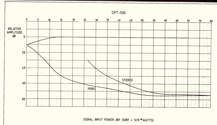
Relative amplitude against signal input power in dBF (0 dBF =  $10^{-16}$ W).
