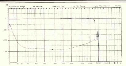
The response of the tuner. Above: the FM section; below: the AM section. The lower trace in the FM graph is channel separation.
