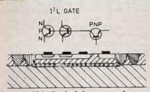
Integrated injection logic in seven mask technology. The region enclosed by  $N^*$  regions comprises the injection logic gate structure.
