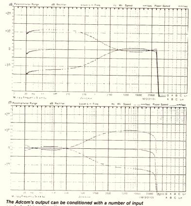
controls. At top: the effect of tone control max boost and cut between 2 Hz and 200 Hz. Above is the same thing but shown between 200 Hz and 200 kHz. Below is shown the effect of low and hi cut filters. At bottom is the effect of the contour control. In all cases the vertical axis covers 50 dB.
