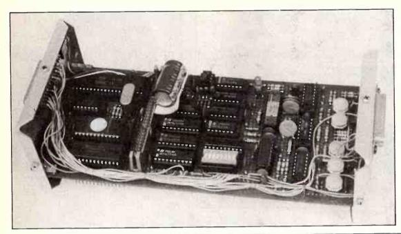
Figure 3: Top: the prototype board of the mark one. Below is the reverse of the same board. It was constructed using wire wrap. An invitation for rats to set up shop, perhaps!
