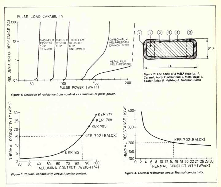
important ones. The density, average grain size and type of minority phase present are also important. Figure 3 shows the thermal conductivity versus the alumina content.
