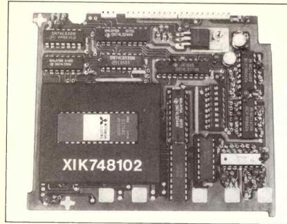
Figure 4: The first production version of the digitalker
