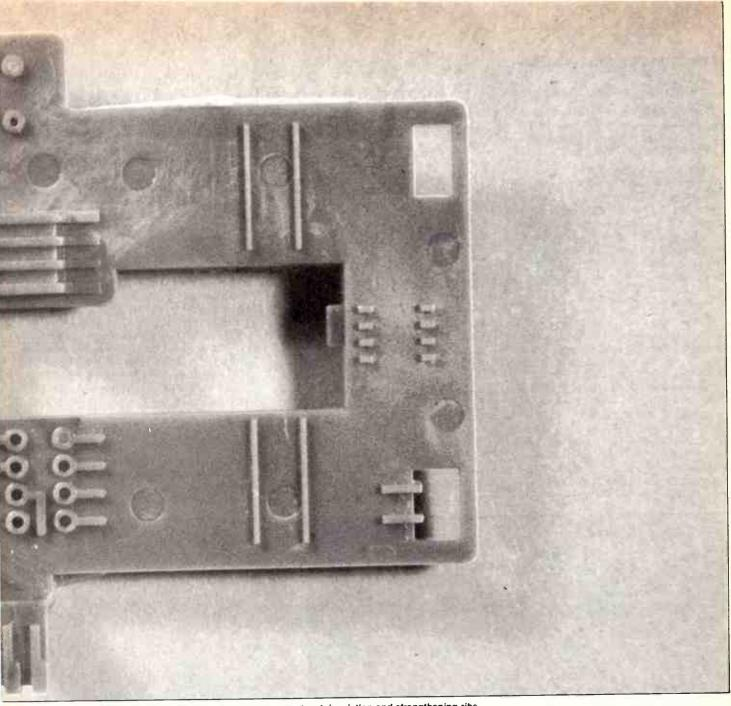
Moulded board substrate showing detailed standups, tracks of insulation and strengthening ribs.
