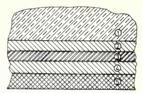
Figure 7. Cross section through the solder contact.
