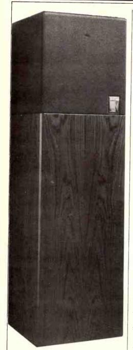
Kef Reference Series 107 Speakers Among the classiest units on the market the new Kefs 107 Speakers use pairs of 250mm diameter woofers operating in a push pull unit. These drivers have a common rod interconnecting the two magnet systems so that the non linear forces are effectively cancelled. The Kefs also feature an active low level equaliser known as a KUBE.
