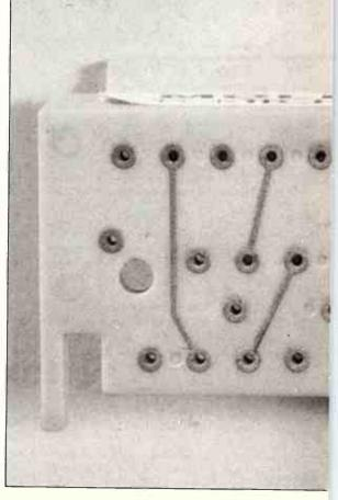
tive plating methods used for FR-4 boards can be used for thermoplastic moulded boards provided they are flat 2-D configurations. The injection moulding materials are all able to give the required 8 to 10 lbs/inch adhesion requirements for conventional boards.
