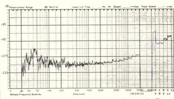
Signal to noise ratio with a one third octave band noise generator. At top reference to a 5mV input. At bottom, a 500 mV input.
