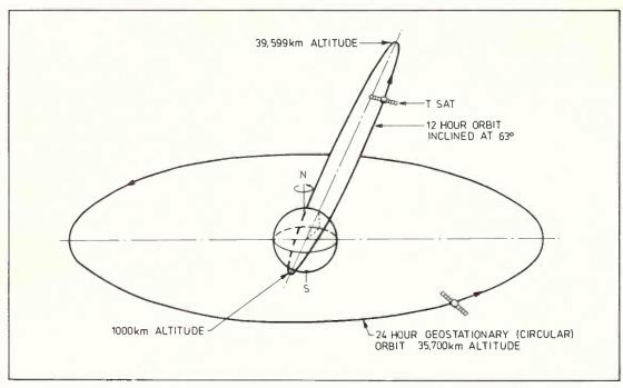
The Molniya satellite orbit compared with the geostationary (circular) orbit.
