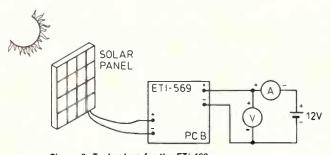
Figure 2: Test set up for the ET/-469.
