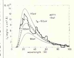
Figure 6: Measured spectrum of the radiation in the gold cavity is observed through a diagnostic hole. For comparison ideal Planckian spectra of different temperatures are shown. The dashed Planckian with a temperature of 102 eV fits the measured spectrum best.
