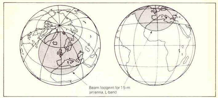
Comparison of coverage by (left) a Molniya orbit and (right) a geostationary orbit.
