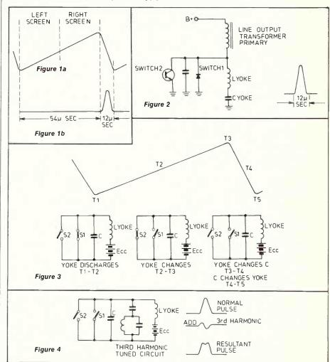
The voltages involved are very large. As a rule of thumb, the maximum induced voltages across C, S1 and S2 will be 8 to 10 times the supply voltage. It is usual to add 10% to 15% for mains variations and increases in horizontal frequency.
