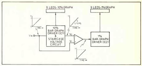
Figure 1: ETI 180 block diagram.
