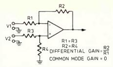
Figure 4: Differential amplifier implemented with an op-amp.
