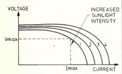
Figure 1: Voltage and current output at various light intensities.
