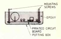
Figure 3: Schematic diagram of the potted box.
