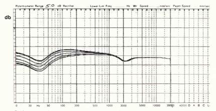
Performance of the Kube Law Frequency Equaliser. The top graph shows low end boost with Q=0.3. The middle graph shows the effect of changing the Q and at bottom is a Q of 0.5 with differing contour settings.
