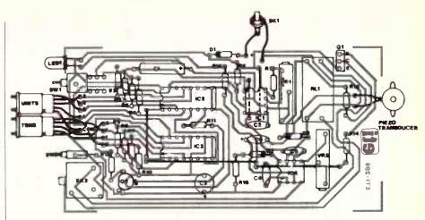
Adjust VR1 to approximately 6k2. Mount IC4, C4, C6, C5, VR2, C3, LED1, R15 and R16. Check the polarity of C6 and LED1. Attach the piezo transducer. Use long leads to do this. Power up the board and place a digital watch over the transducer. Activate the alarm. Adjust VR2 until
