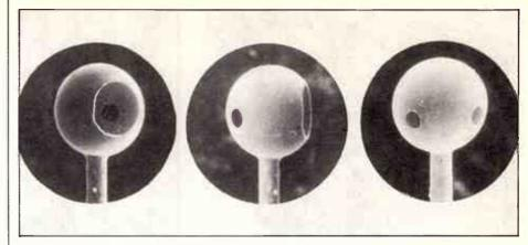
Figure 5: Three different views of a spherical gold cavity (diameter 280 µm, wall thickness 2 µm). The laser radiation is injected through the large hole. The radiation inside the cavity is observed through the two smaller diagnostic holes.
