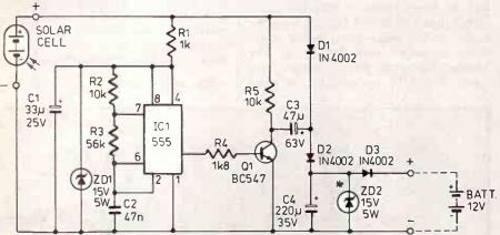
When the solar cell is creating a voltage much greater than the battery, the typical charge-type situation, then the circuit may be considered to consist merely of the solar cell and the battery. Current will flow from the solar cell into the battery. All the other components are present solely because this situation does not always pertain.
