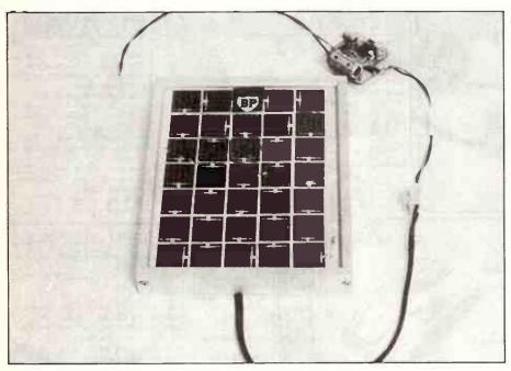
THE ETI-569 Solar Charger is designed to charge any standard 12 V lead acid car battery in any area where mains power is unavailable. It is ideal for remote data acquisition stations, caravans and boats.
