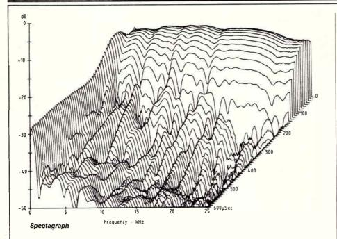
distortion at 1 kHz was somewhat higher at 3.3% and again symptomatic of the colouration at that frequency. The high frequency distortion is quite low and the tweeter's performance is extremely good.
